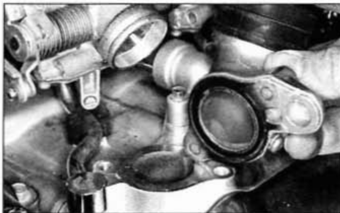
8.8b Pull the intake tubes off the carburetors; on installation, use a new O-ring between the intake tube and cylinder head
