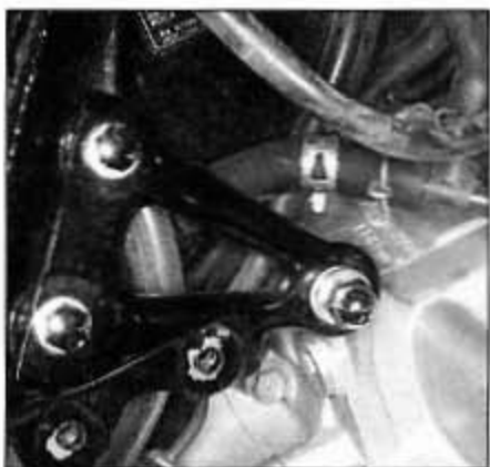
5.20a Remove the two bolts and cap nut from the right engine mount . . .
