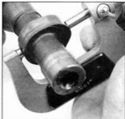
9.9b Measure the height of the camshaft lobes with a micrometer
