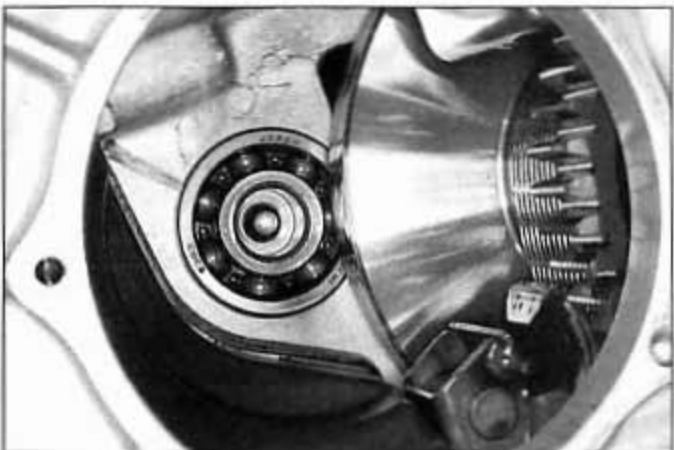
31.7 The drive unit's front bearing is mounted inside the crankcase
