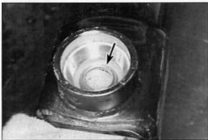
13.5 Replace the outer races and bearings as a set if either outer race is worn; don't forget to reinstall the inner grease retainers (arrow)
