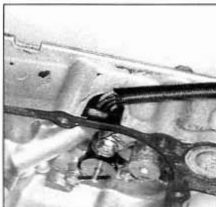
18.9 The wiring harness grommet fits under the gasket like this
