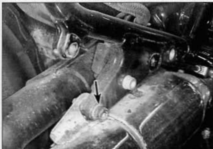
13.3 Remove the muffer mounting bolt (arrow)
