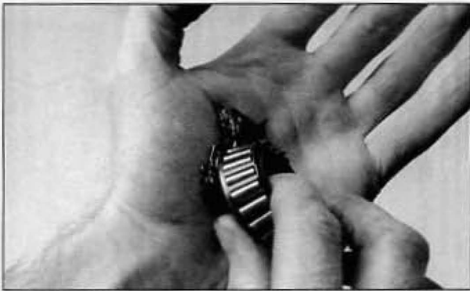
7.17 Work the grease completely into the rollers or balls
