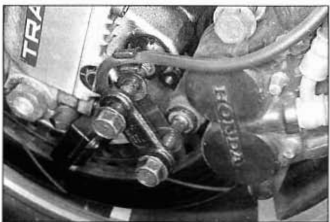
2.11 Be sure this plate (and shim, if equipped) is in position when reinstalling a front caliper
