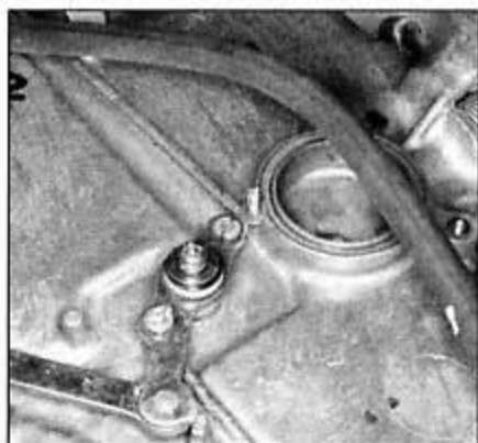
9.4 Remove the cotter pins and washer to free each choke rod from its pivot; there's a second washer on the other side of the bushing
