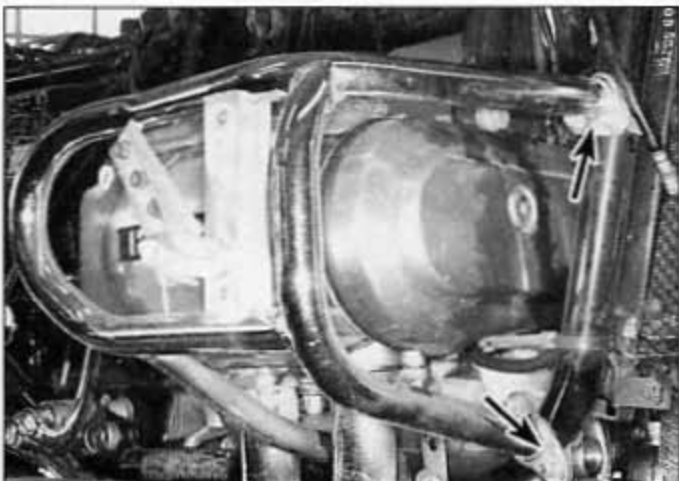
7.3 The engine guards are held to the frame by a pair of clamps (arrows); under the bike, they're attached to each other
