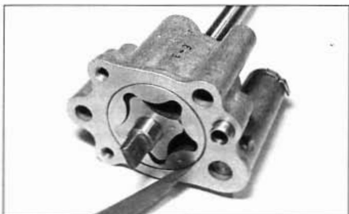
17.9b . . . and between the inner and outer rotors
