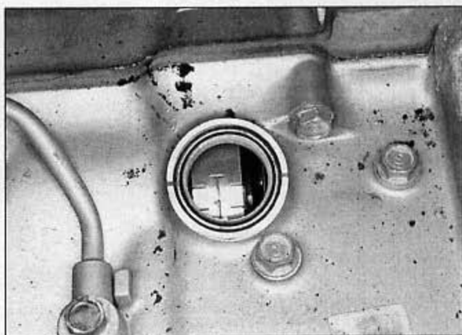
7.4a With the engine at top dead center on its compression stroke, the line next to the T-1 mark on the crankshaft pulley will align with the lines in the crankcase ...
