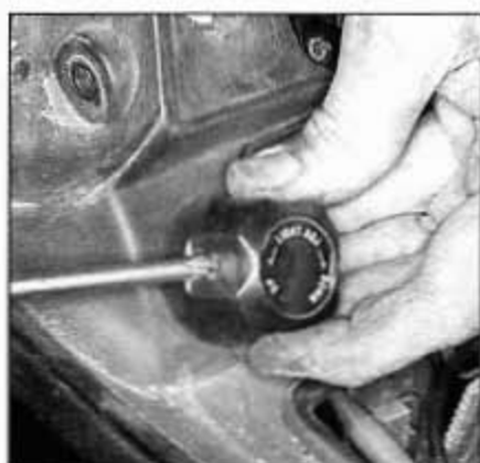
7.8a Undo the screw and pull off the vertical aiming knob ...
