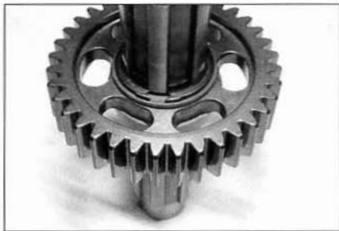
33.13a Remove the second gear snap-ring; this snap-ring is installed correctly, with its gap centered on a gap in the countershaft splines
