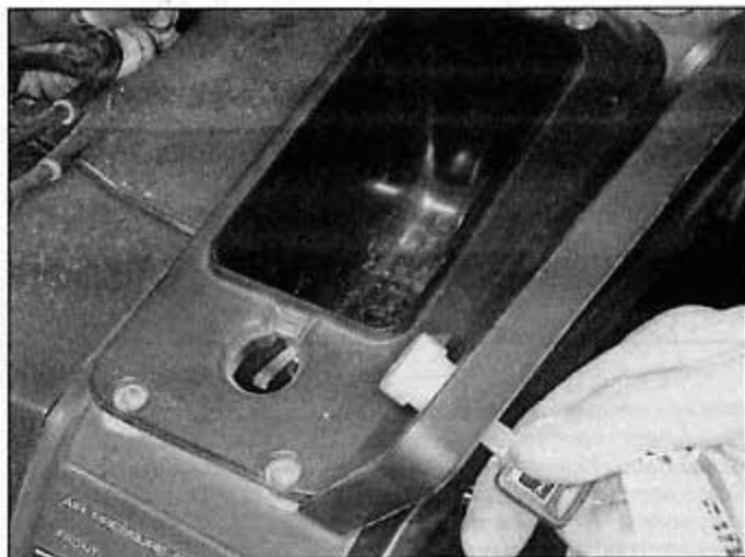
3.1a Open the right fairing pocket with the key and remove its mounting screws
