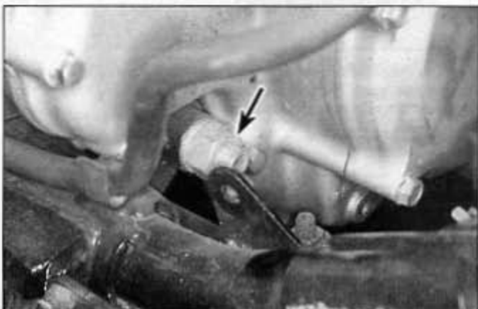
5.18a On the left side of the bike, remove the lower engine-to-subframe nut/bolt (shown) and the lower engine-to-subframe bolt that's below the cylinder head
