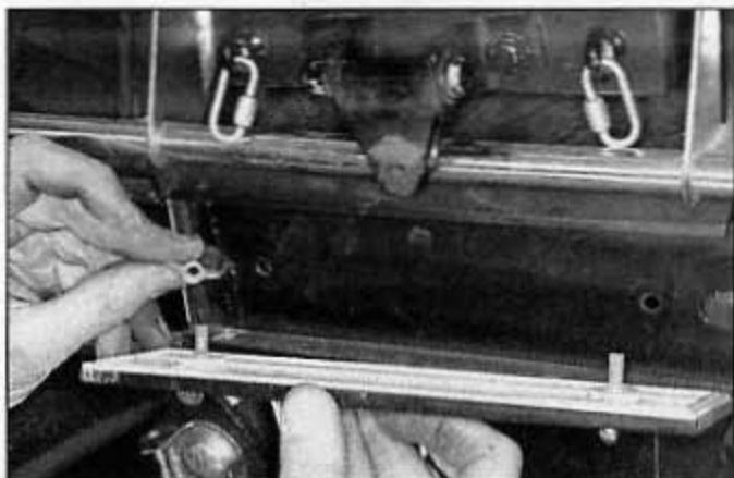
12.1 Remove the wing nuts from behind the reflector and take it off
