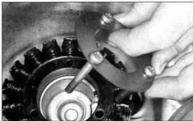
30.3 Remove the screws and plate (you'll need an impact driver) to free the stator from the housing
