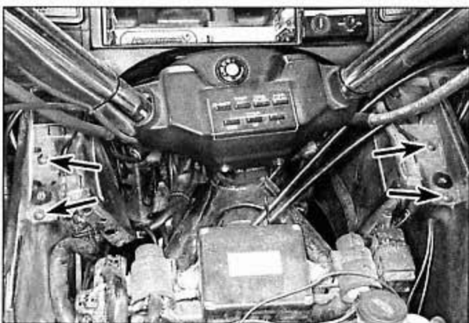
11.2a Remove the screws to detach the harness retainer on each side of the bike (arrows)
