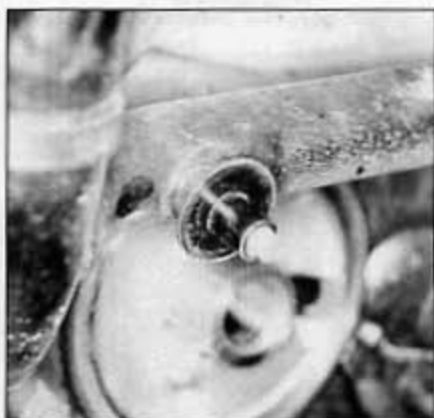
7.7 Check the collars and mounting studs for corrosion or damage
