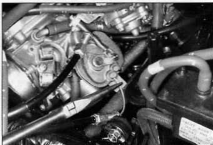
12.2b Rotate the cable to align it with its pulley slot, then slide the cable end sideways out of the pulley
