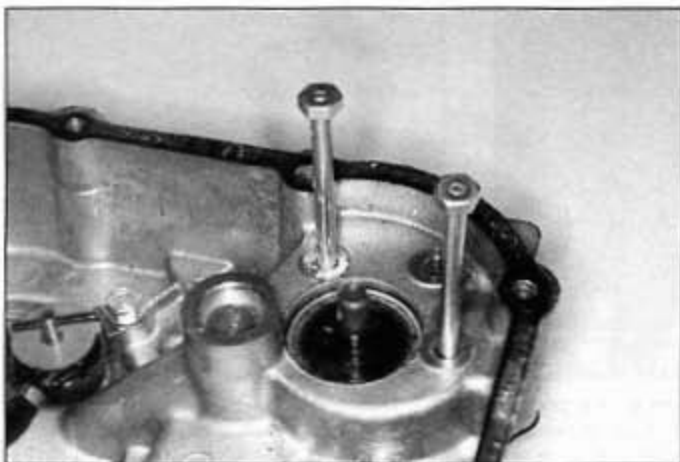
8.8b Thread a pair of long bolts into two of the bolt holes . . .
