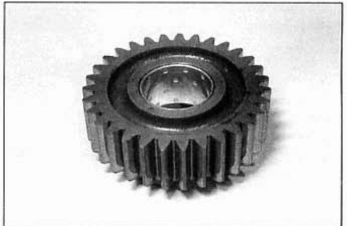
33.6 1984 through 1986 models use this permanent fourth gear bushing; 1987 models use a separate bushing
