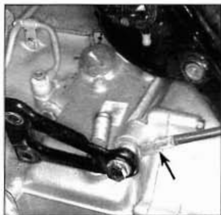
5.20c . . . the through-bolt, which connects the left and right engine mounts, secures a ground cable (arrow) on the left side
