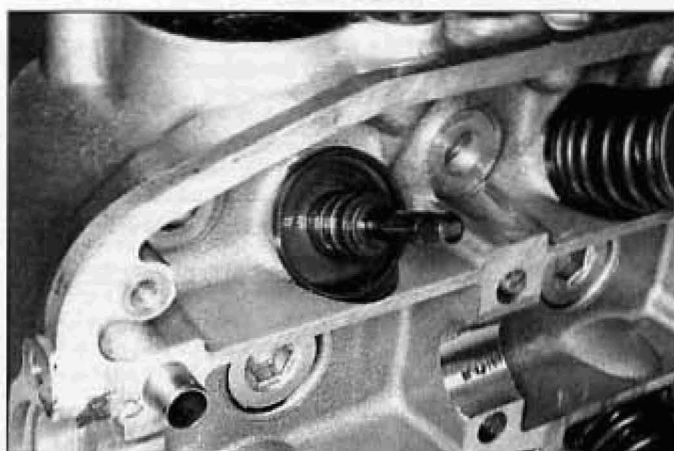
12.28 Install the lower retainers and seals on the head
