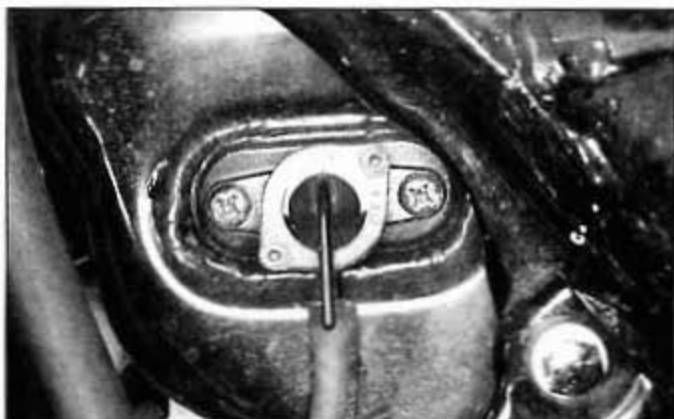
2.11 Remove two screws and take the fuel tap off the tank; use new O-rings on installation
