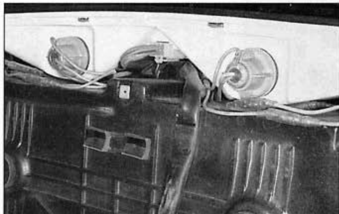
9.11 Aspencade rear brake lights are accessible from below
