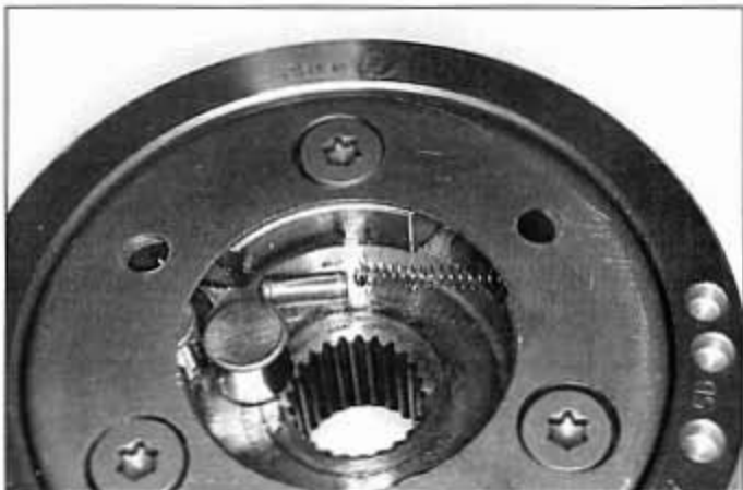
30.10 The springs fit into holes in the starter clutch; the pins fit over the springs and secure the rollers in their holes
