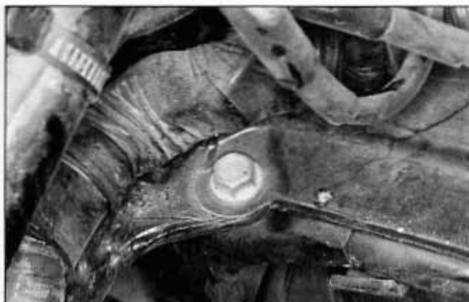
5.17a Remove the front mount upper bolts (there's one on each side of the bike) . . .
