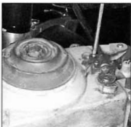
7.8d Undo the screws and detach the aiming cables from the housing
