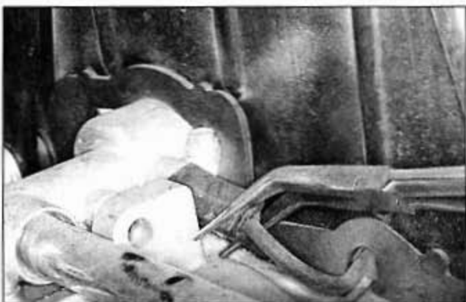
5.4a Pull the connector off the coolant temperature sender; note how the wiring harness is routed through a notch in the radiator shroud
