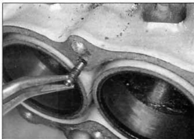
10.12 Lift the oil orifice out of its passage; its inner O-ring is smaller than the outer one
