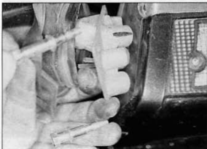
9.2 ... The screws are different lengths; on installation, install the top screw first
