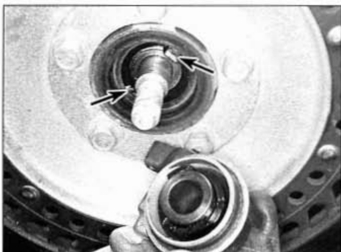
12.12a On installation, make sure the speedometer coupling lugs (arrows) engage the notches in the drive unit
