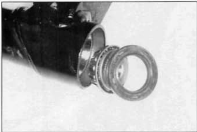
13.3b Remove the seal and bearing
