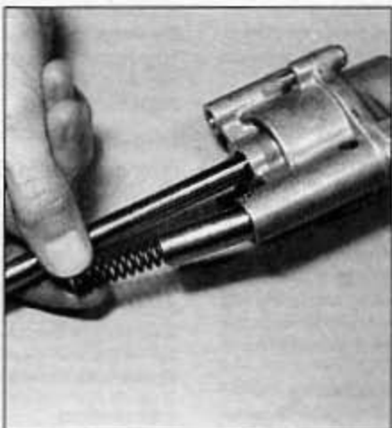
19.2g Pull out the spring and relief valve and check the valve for wear or damage
