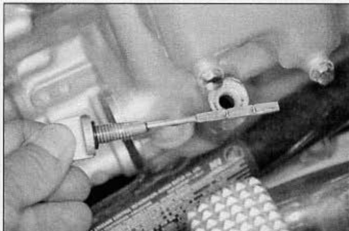
3.3 Check oil level on the dipstick; it should be between the Minimum and Maximum marks
