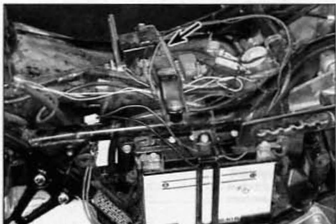
2.9 Unbolt the crosspiece (arrow) and lift it off the frame
