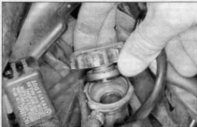
27.7 Inspect both cap gaskets
