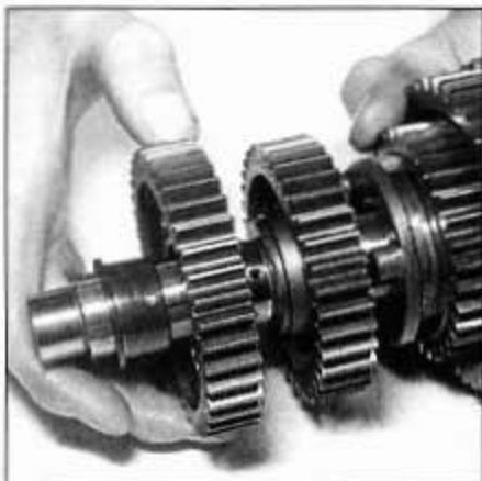
33.13b Slide off the bushing and second gear; on installation, the bushing oil hole must align with the hole in the shaft
