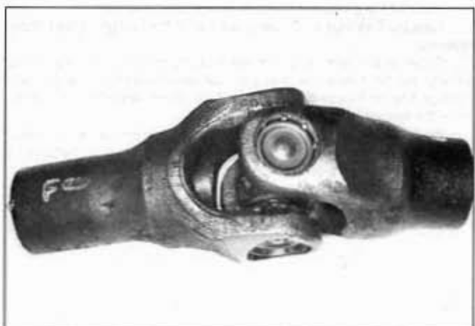
12.10 The long end of the universal joint, which is stamped with an F, goes toward the engine
