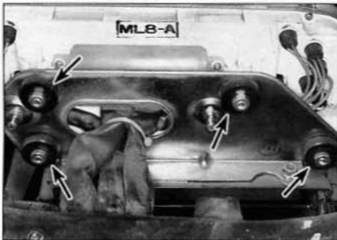
23.1 Remove the mounting nuts and bushings (arrows) and separate the cluster from the bracket
