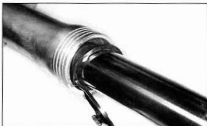
5.5 Remove the retainer from its bore with snap-ring pliers
