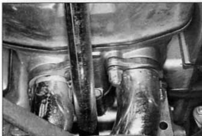
13.2 Remove the nuts and retainers and lower the pipes away from the cylinder head
