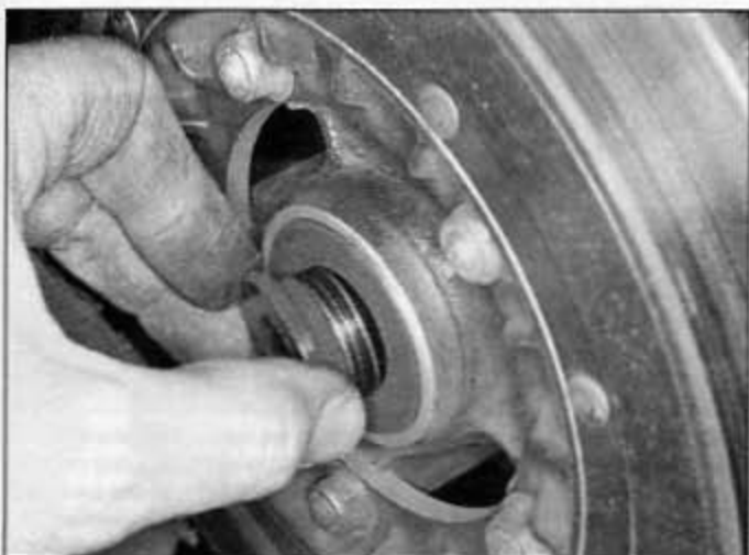
13.8 Remove a second collar from the left side of the wheel
