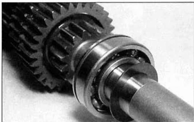
33.4a Remove the thrust washer from the mainshaft
