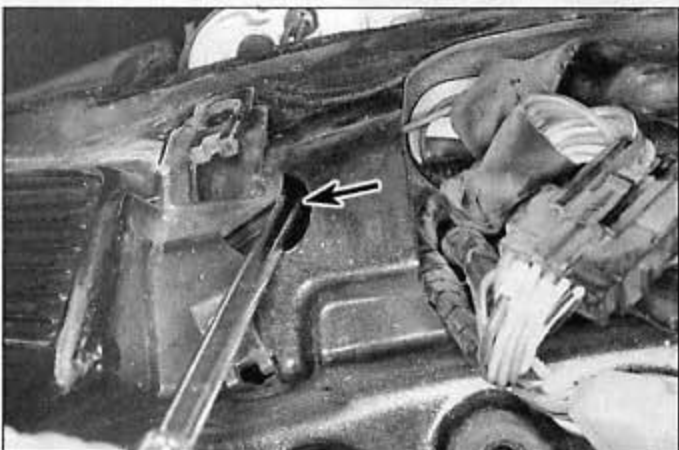
21.9b . . . and the upper nuts (arrow) to free the cluster, then lift it up and unplug the electrical connectors
