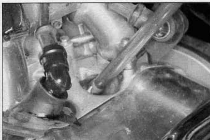
16.8 Threading the plugs in with a piece of hose will save time and prevent damage
