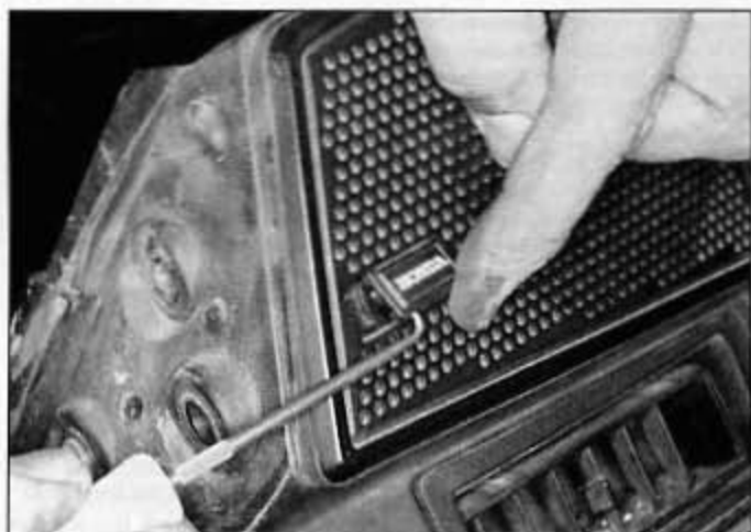
32.3 Pry up the speaker cover trim with a pointed tool, remove the cover screw and take off the cover . . .
