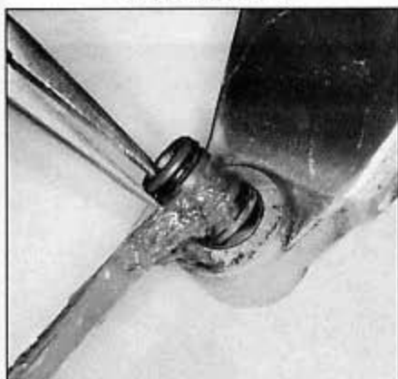
5.17b Install new O-rings and coat the collar liberally with grease
