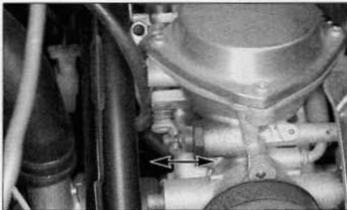
9.7 Measure the stroke of the choke valves
