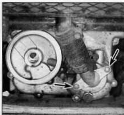
7.5b Loosen the lower hose clamp screws and remove the water pump cover bolts (arrows)
