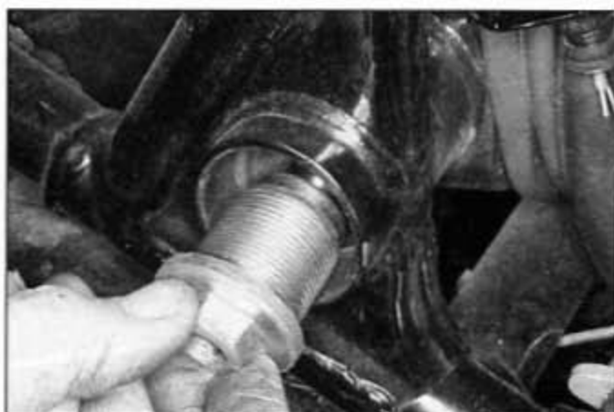
12.7b . . . and unscrew the right pivot bolt with a socket; on installation, grease the pivot bolt tips and make sure they engage the swingarm bearings
