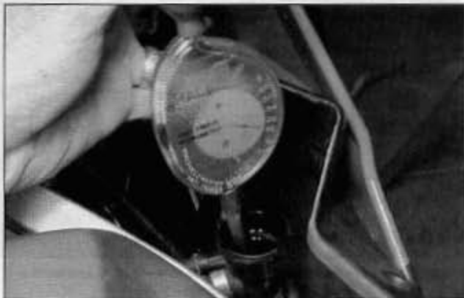
27.8 An antifreeze hydrometer is helpful in determining the condition of the coolant
