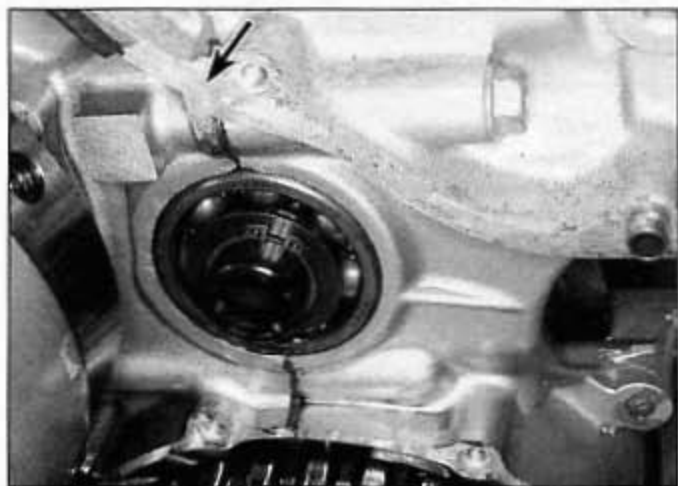
15.10 Apply a dab of sealant at each point where the gasket crosses a crankcase seam (arrow)
