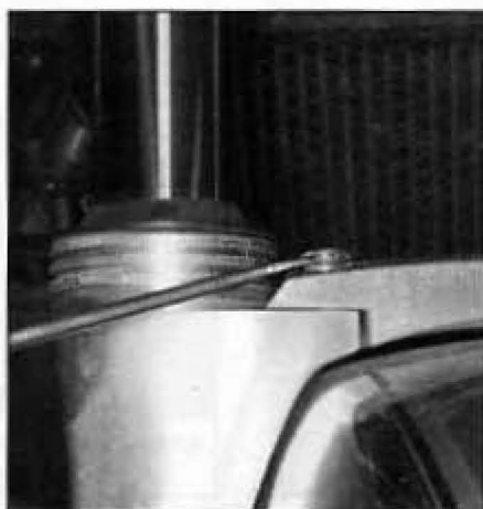
4.5a Pry the trim caps out of the fork brace bolts . . .
