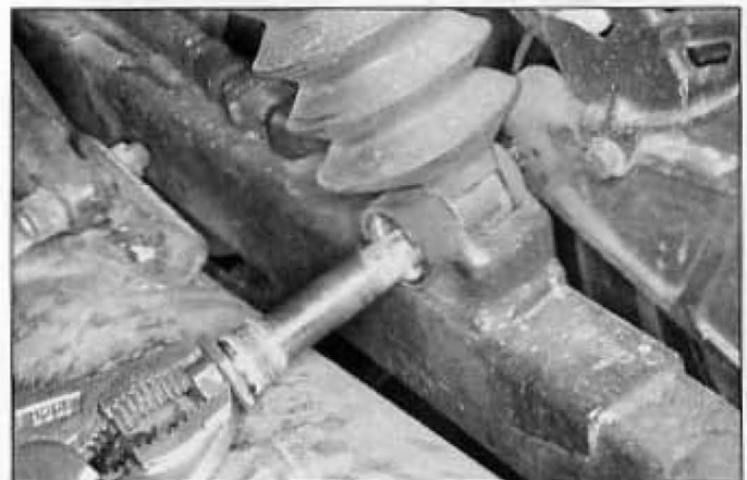
8.4a The left lower mounting bolt is threaded next to its head
