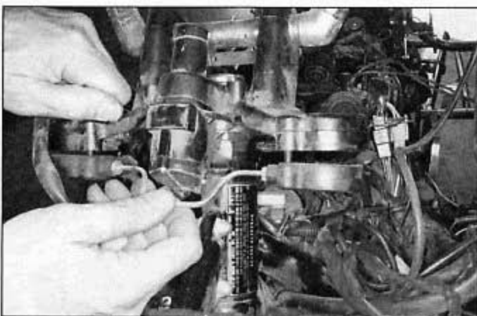
4.9d Remove the screws and lower the air equalizer away from the upper triple clamp
