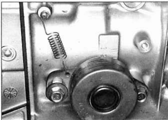
7.19b ... and the right spring is installed like this
