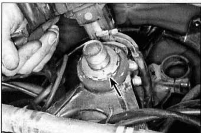
6.3c Lift the upper triple clamp off the steering stem; bend back the lockwasher tabs (arrow), unscrew the locknut . . .
