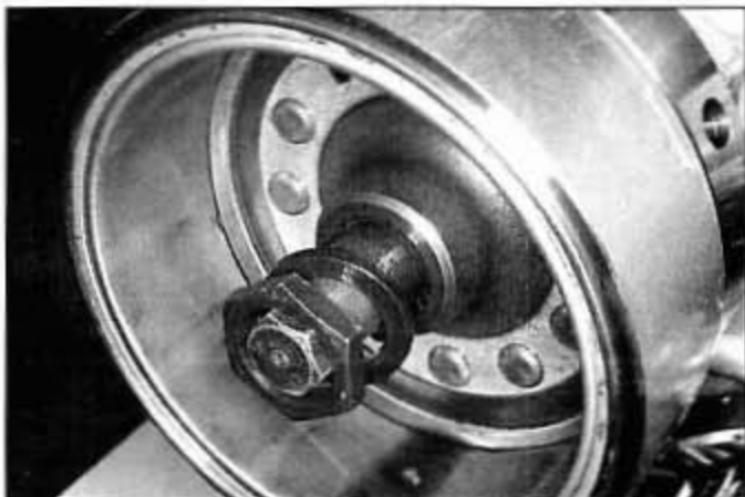
30.11 Don't forget the washer when reinstalling the rotor nut
