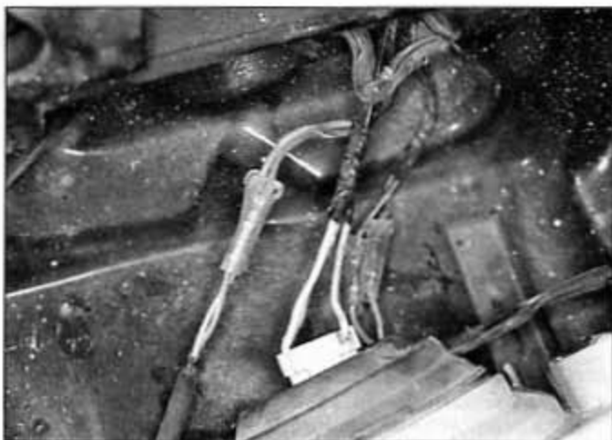
7.5a ... then pull the assembly forward and unplug its electrical connectors
