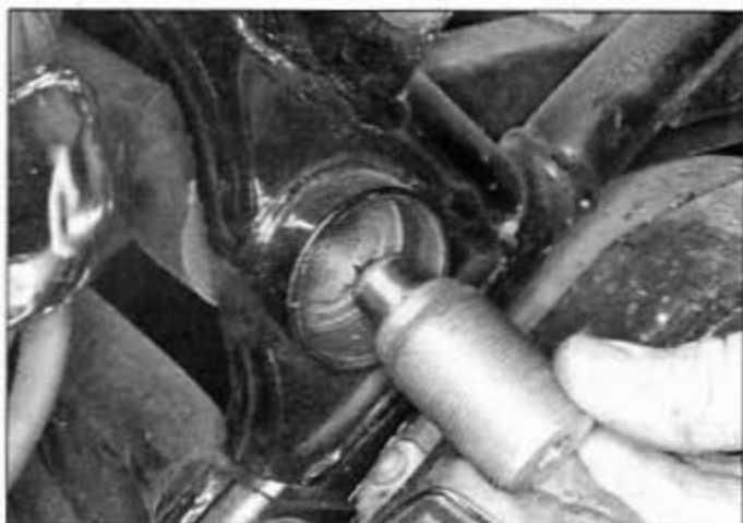
12.7a Unscrew the left pivot bolt with an Allen bolt bit . . .
