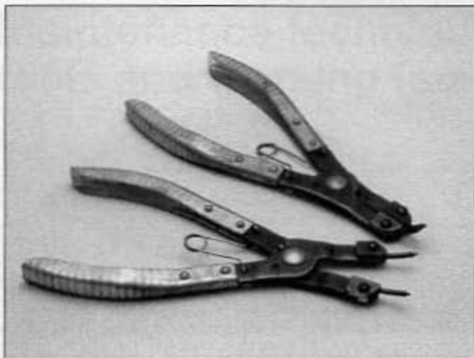
Snap-ring pliers (top - external; bottom - internal)
