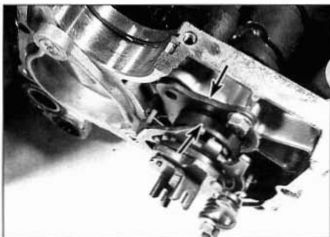
20.13 Remove the drum center (lower arrow) and the bearing retainer (upper arrow) for access to the bearing
