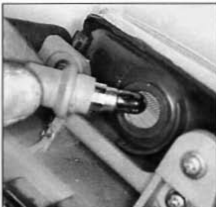
7.9b . . . pull the socket out of the housing, then pull the bulb out of the socket
