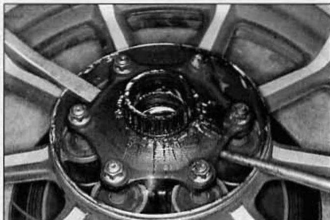
10.7 Pry the coupling evenly from the wheel
