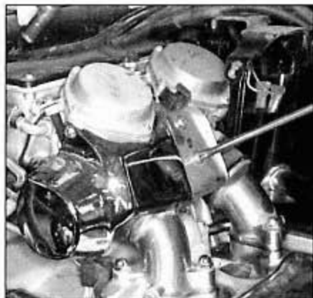
8.5 Remove the carburetor covers
