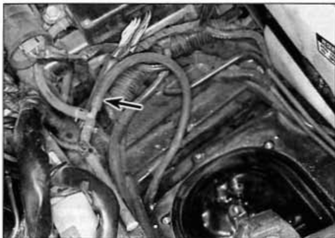
5.3 Disconnect the vacuum line (arrow) at the T-fitting
