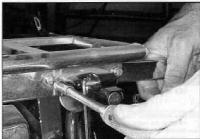
14.2 Unbolt the antenna bracket from the trunk bracket
