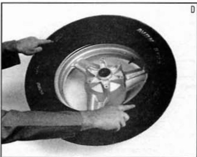
D Before installing, ensure that tire is suitable for wheel. Take note of any sidewall markings such as direction of rotation arrows.
