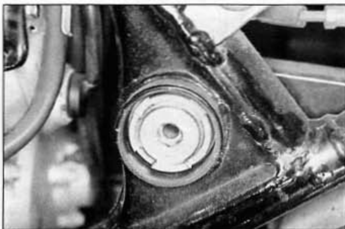
12.6a A special tool is needed to fit the slots in the left pivot's locknut
