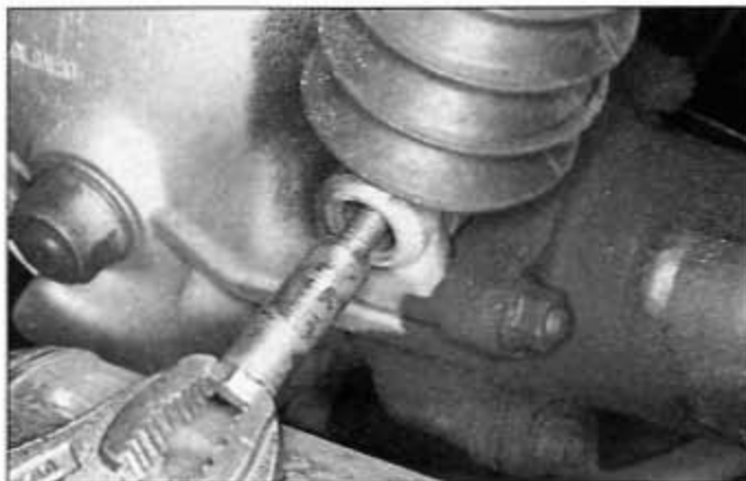
8.4b The right lower mounting bolt is threaded on its end
