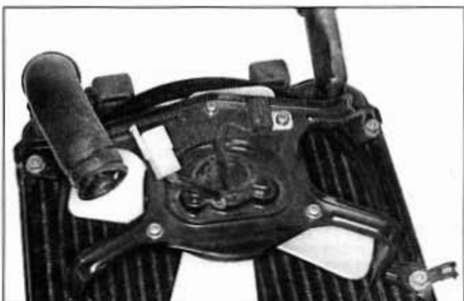
4.7 Four hex-head screws secure the fan motor bracket to the radiator; three Phillips screws secure the fan motor to the bracket
