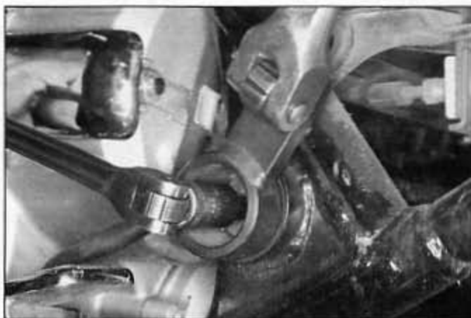
12.6b Place a breaker bar in the hole of the special tool; hold the pivot bolt with an Allen bolt bit while loosening the locknut
