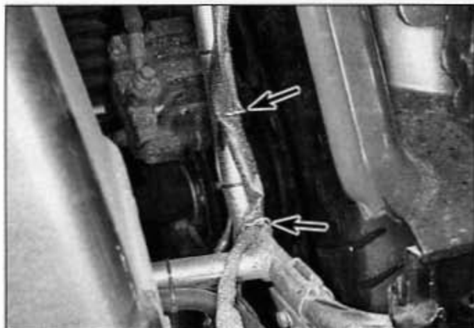
12.4 Lift the saddlebag part way off, detach the harness clips (arrows) and unplug the connector
