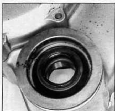
15.9 Pry out the output shaft seal and tap in a new one
