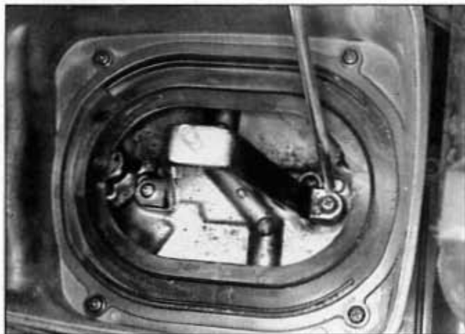
5.4 Remove four screws to detach the housing and two screws to detach the element bracket
