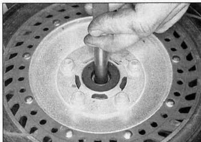
14.5c Pass the wedge end of the rod through the hub into the split portion
