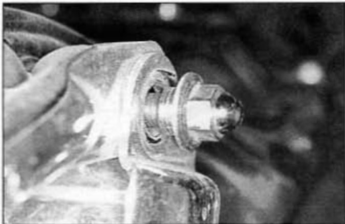
8.5a The shoulder of the upper nut fits inside the cover
