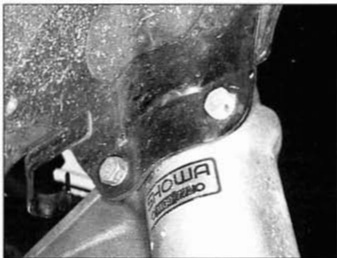
5.2 The front fender is bolted to the fork legs from the inside
