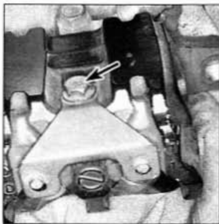
2.5a Undo the retainer bolt (arrow), lift off the retainer and pull out the pins ...
