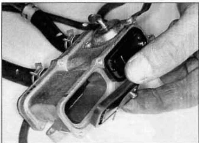
14.5c . . . and take the reeds out of the case
