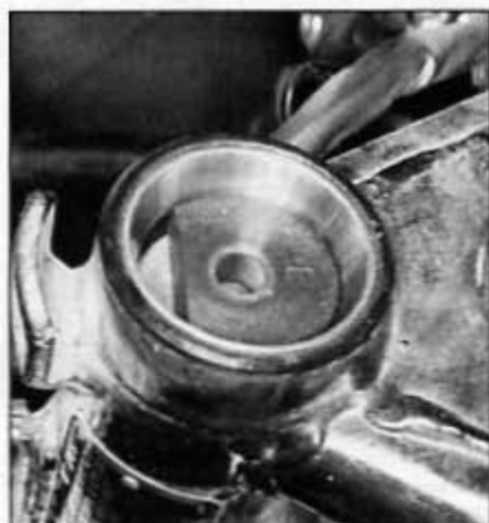
7.11a This Honda tool fits into the upper bearing race; tapping the tool upward from below will push the race out
