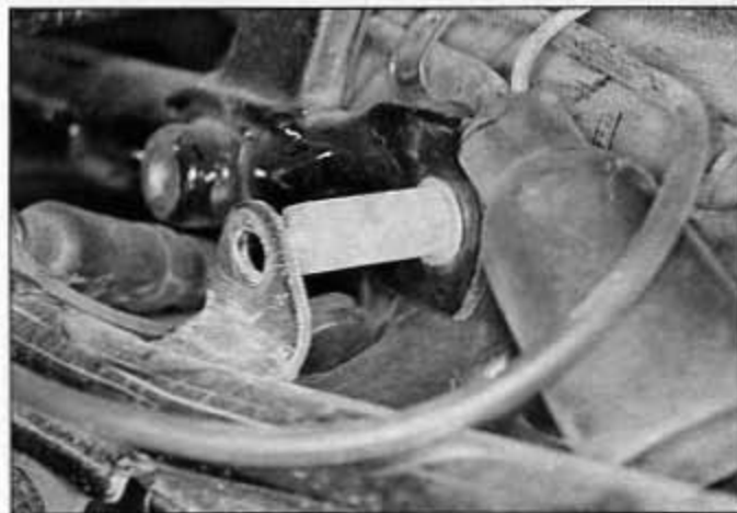
14.7 The upper bolt passes through the bracket into the fender bolt on each side
