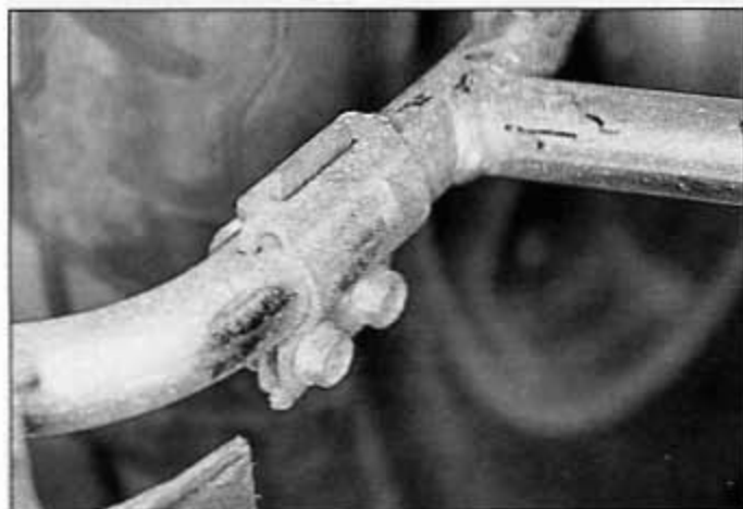
14.5 The rear bumper is secured at each end by a clamp
