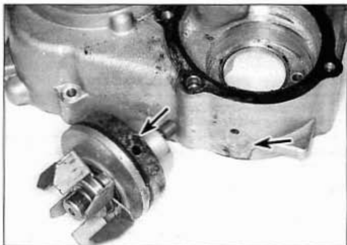
8.9 Stains around the telltale hole and corrosion on the pump body indicate that it's time for a new water pump
