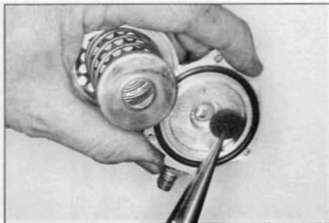
9.9 This small filter fits in a bore in the cover
