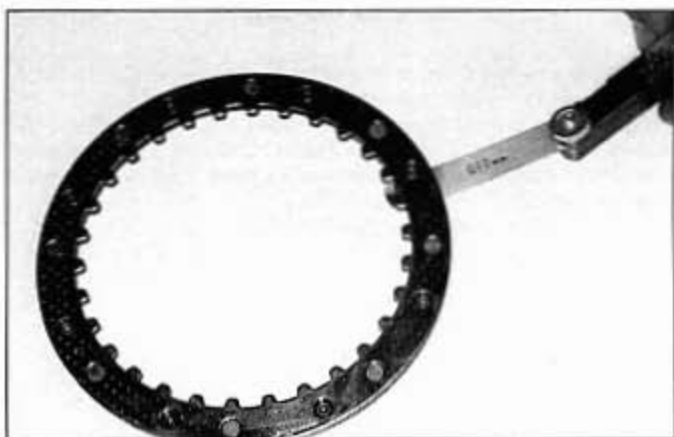
14.20a Check the clutch damper for warpage . . .
