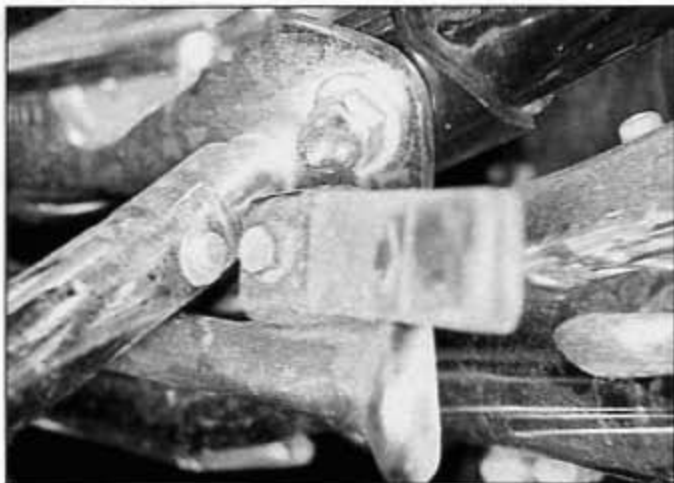
16.1b The sidestand rubber tip can be replaced separately if it's worn
