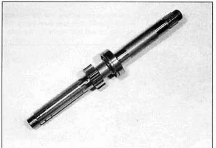
33.9 First gear is integral with the mainshaft; replace the bearing if it's worn or damaged
