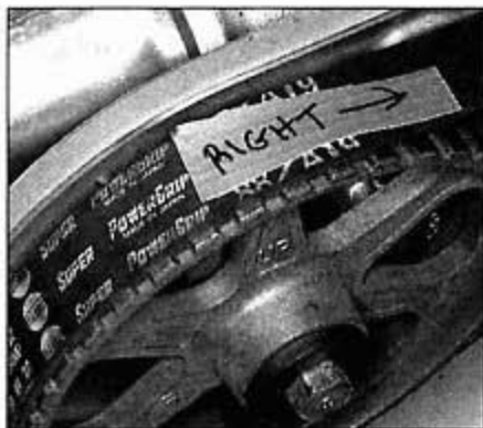
7.5a Label each belt with Left or Right marks and an arrow indicating direction of rotation
