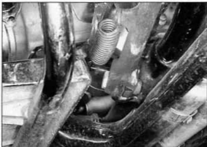
16.1a Unhook the spring and remove the pivot bolt to remove the sidestand
