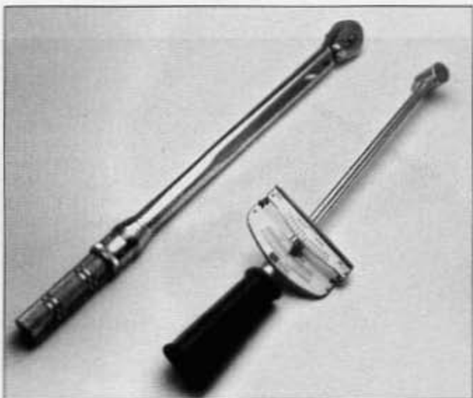
Torque wrenches (left - click; right - beam type)
