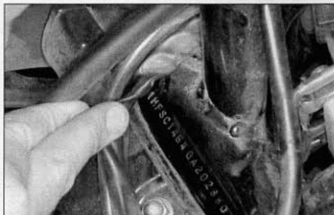
The frame number is stamped in the steering head . . .
