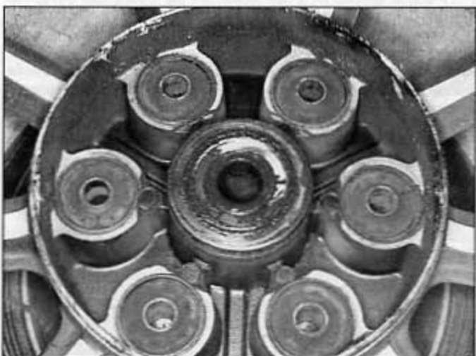
13.12 The wheel must be replaced if these dampers are worn enough to allow lash in the driveline
