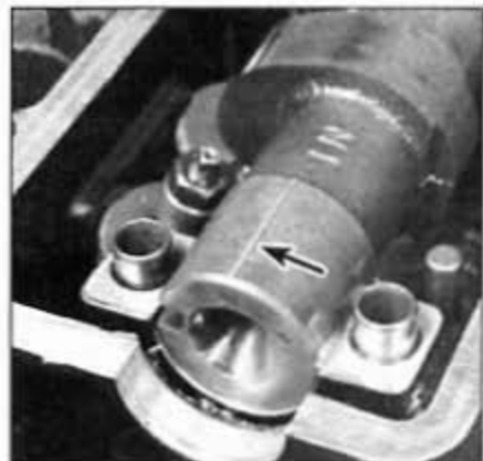
9.11 Lay a strip of Plastigage lengthwise along each journal
