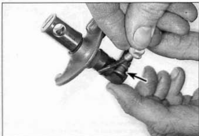
9.26b . . . the spring-loaded assist shaft and the lash adjuster (arrow) rotate the rocker shaft, moving the pivot point to eliminate valve clearance
