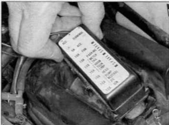
3.21 Move the fuse block aside so it isn't spilled on
