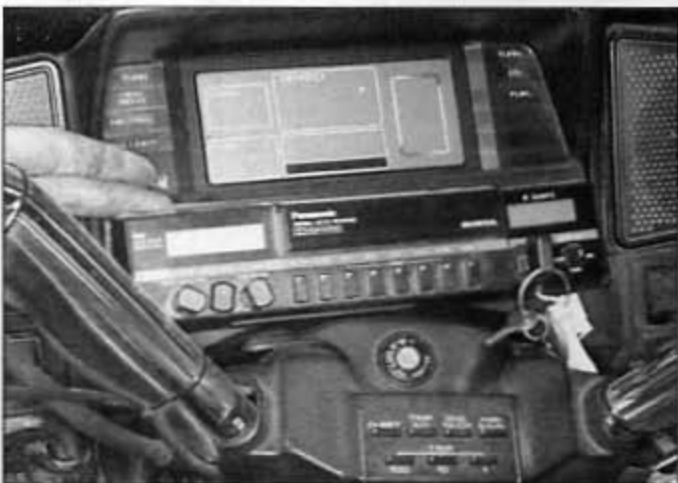
32.1 Unlock the radio with the ignition key . . .
