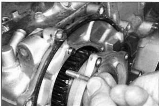
31.3 Pull the drive unit out of the engine; the long bolt goes in the hole with the dowel
