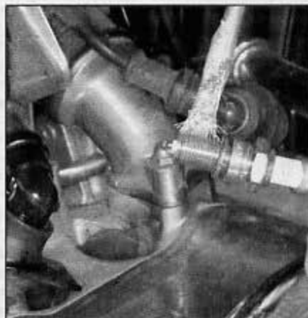
16.7c A small dab of anti-seize compound will make the plugs easier to remove later
