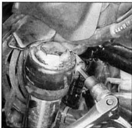
4.9a Loosen the upper triple clamp bolt ...
