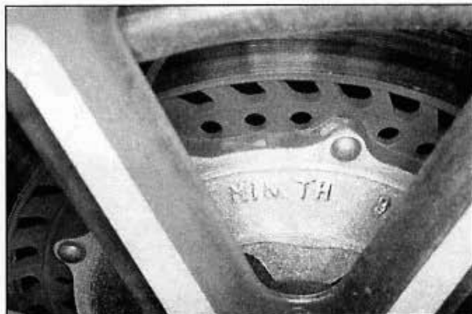
4.4 The minimum thickness is cast into the disc
