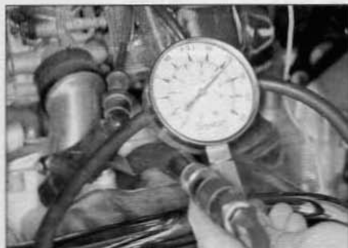
15.8 A compression gauge with a threaded fitting for the spark plug hole is preferred over the type that requires hand pressure to maintain the seal
