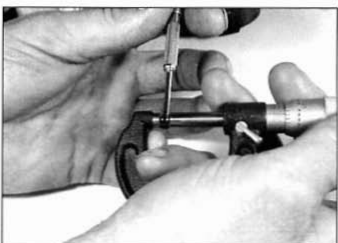
12.16 . . . then measure the small hole gauge with a micrometer
