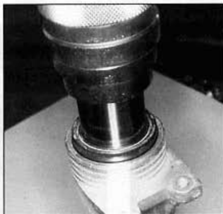
5.23a Drive the bushing and oil seal into the outer fork seal bore like this
