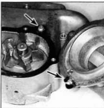
8.6b . . . take the housing off the pump body and locate the dowels (arrows)
