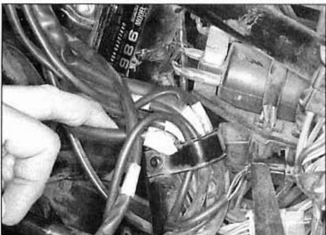
16.11 Free the harness from the retainer and unplug the electrical connector
