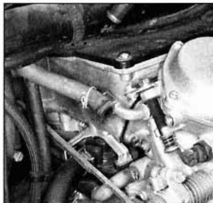
8.7a On California models, disconnect the vent hoses . . .
