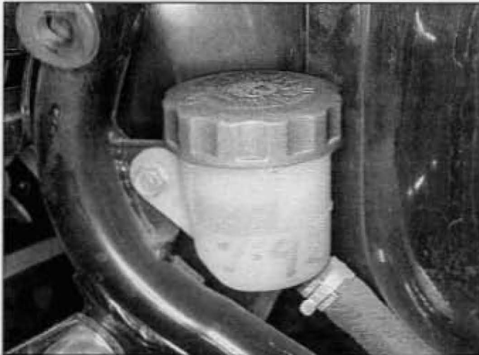
3.15 The fluid level in the rear brake master cylinder can be checked by looking through the plastic reservoir - fluid must be above the Lower mark
