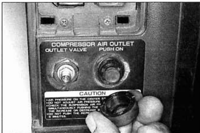
9.4 Unscrew the air outlet knob and the air hose hex nut
