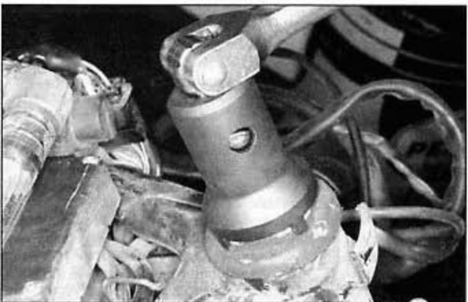
6.4b A socket like this one is needed to torque the adjusting nut accurately; if you use an adjustable spanner, make sure there's no looseness or binding in the steering
