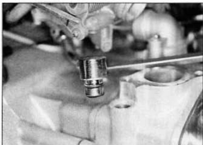
14.3 Pry the air tubes out of the cylinder head; use new O-rings on installation
