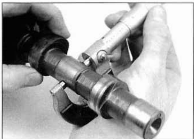
9.14b Measure the cam bearing journal diameter with a micrometer
