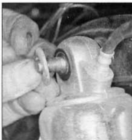
8.5b Remove the washer and slide the shock absorber off the stud
