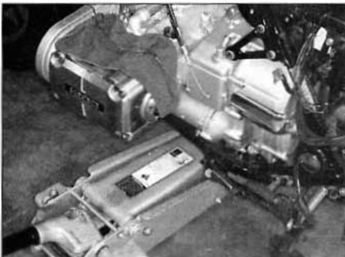
5.22 Use a jack to lower the engine and have an assistant help guide it out of the frame
