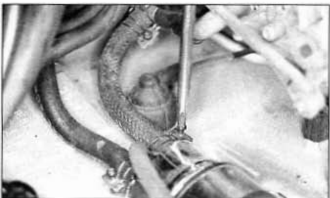
4.3 Undo the fuel pump outlet hose and attach a length of tubing in its place
