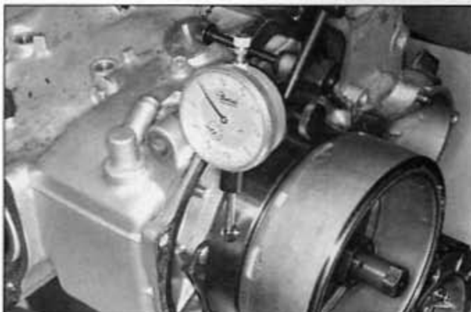
31.21 Correct backlash is necessary to prevent drive unit noise
