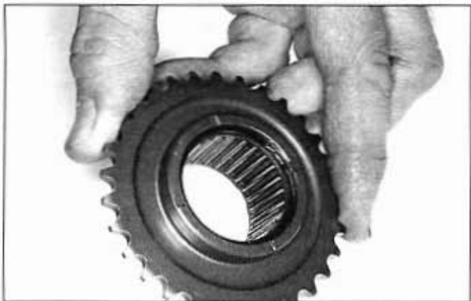
31.5 Because the engine must be removed to get to this bearing, it should be replaced if there's any doubt about its condition
