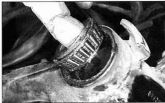
7.7b Lower the steering stem out of the steering head and lift out the upper bearing
