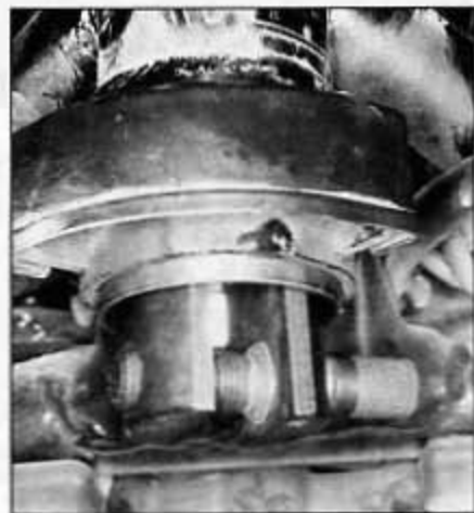
7.11c . . . tapping on the tool from above will push the lower race out (race shown partially removed)
