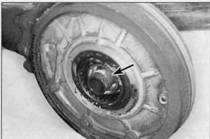
10.5 Check the final drive unit oil seal for leaks; on installation, make sure the spacer (arrow) is in position
