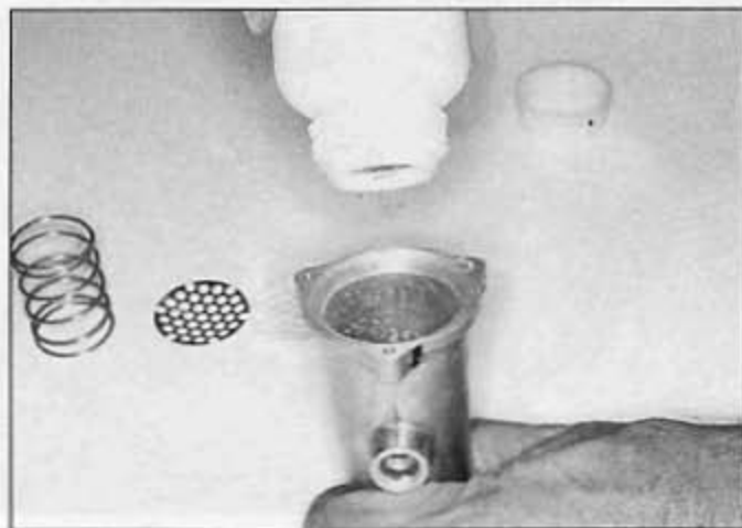
9.13 Pour the desiccant into the drier body (it's pre-measured)
