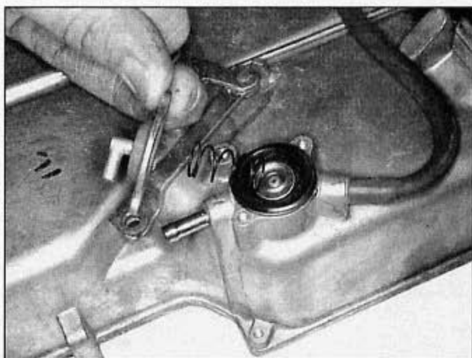
14.5f The slow air cutoff valve spring and diaphragm are beneath this cover
