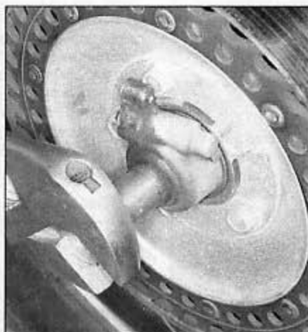
12.5b . . . and remove the axle nut with another
