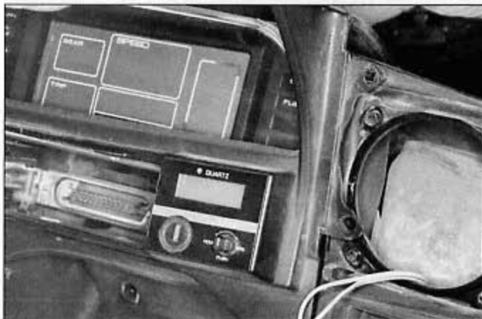
21.7a Remove the mounting screws at each end of the cluster trim cover . . .
