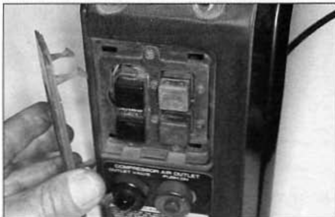
9.3a Carefully pry the cover loose from the switch panel . . .
