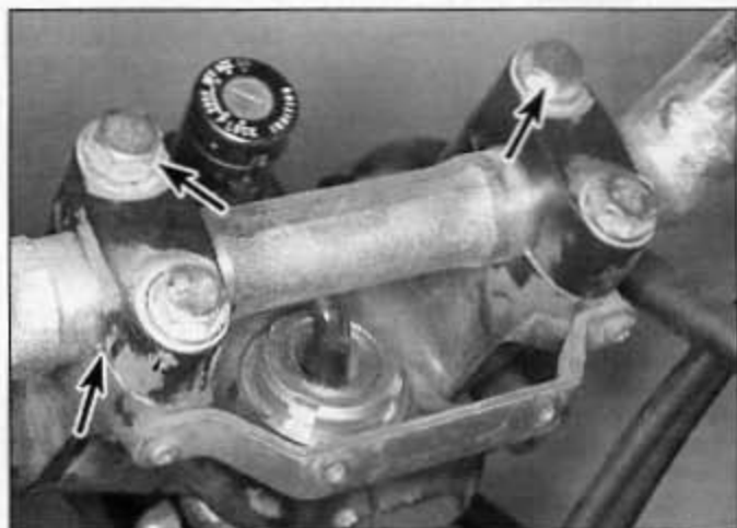
2.2 Align the punch mark in the handlebar (lower arrow) with the lower rear corner of the left bracket; install the clamps with their punch marks forward (upper arrows)
