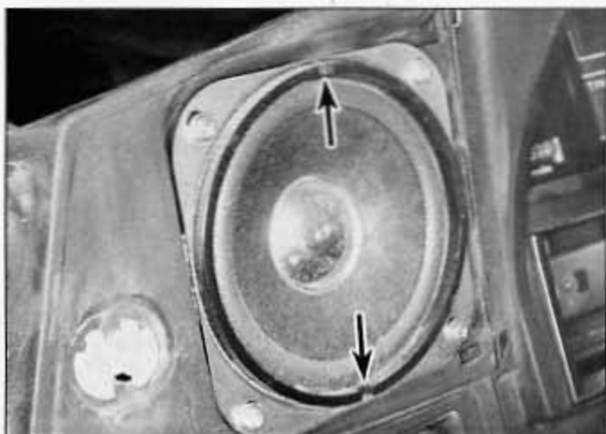
32.4 . . . to expose the speaker screws; the drain slots (arrows) go at the top and bottom on installation
