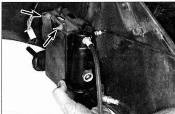
9.5b ... and the drier assembly; when installed, the drier assembly fits on the other side of the panel shown. Its rubber retainers (arrows) ...
