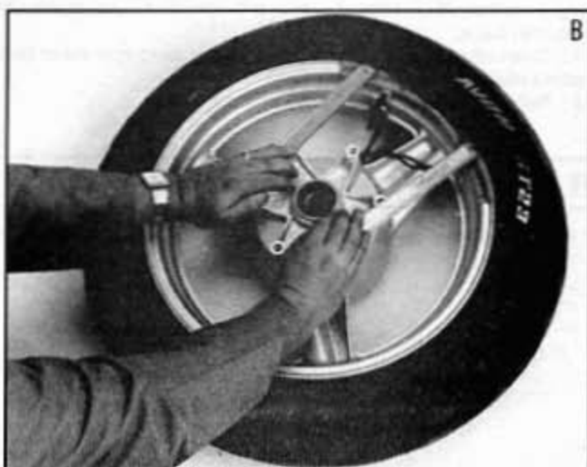
B Use two levers to work bead over edge of rim. Note use of rim protectors.
