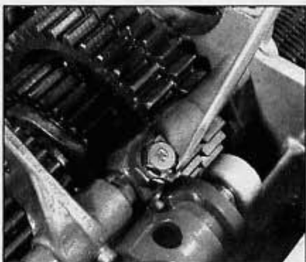
31.3d Bend back the lockwasher tab and remove the bolt from the fork and shaft
