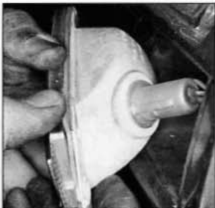
9.1 Take the lens and gasket off the housing for access to the bulb
