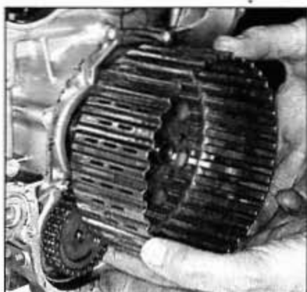
14.11b . . . and pull the clutch housing off, together with the oil pump sprocket and drive chain
