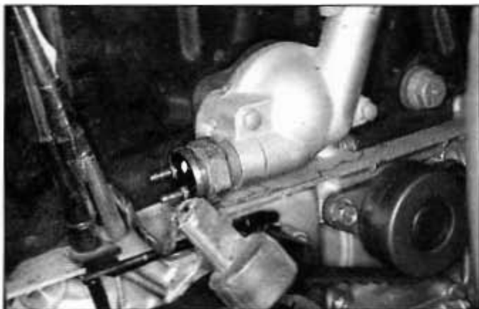
4.4b Pull back the boot and unplug the connector to expose the fan switch
