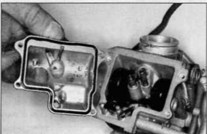
10.2b Remove the screws and take off the float chamber cover; on assembly, use a new O-ring and make sure the dowels are in position
