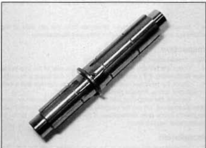
33.13k ... must align with the oil hole in the shaft
