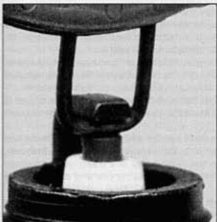
16.7a Spark plug manufacturers recommend using a wire type gauge when checking the gap - if the wire doesn't slide between the electrodes with a slight drag, adjustment is required
