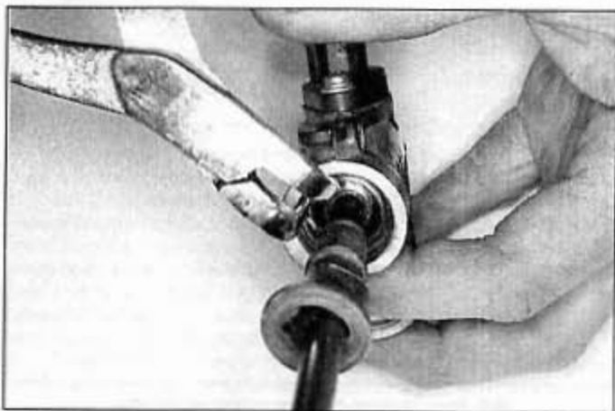
6.10 Remove the snap-ring from the cylinder bore
