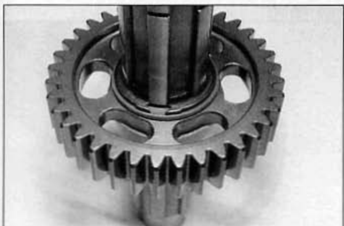
33.13h Remove the third gear snap-ring; on installation, center the snap-ring gap on a gap between the shaft splines
