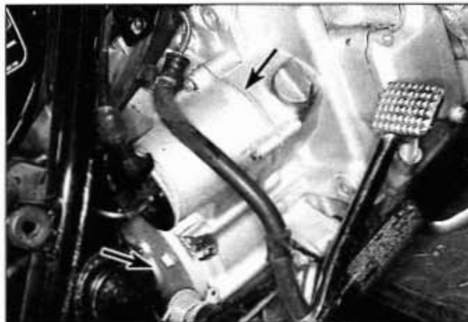
14.4 All clutch components except the housing can be reached by removing the clutch cover (left arrow) with the engine in the frame; to remove the clutch housing, you'll need to remove the engine and the rear crankcase cover (right arrow)
