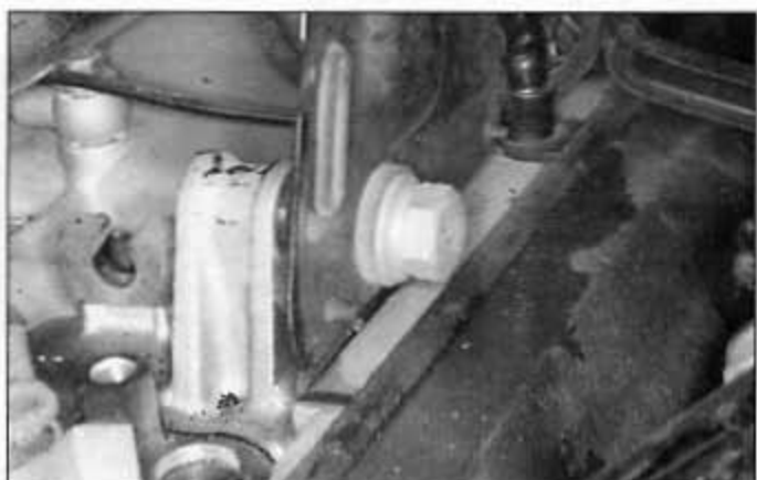
5.17b . . . and the front mount lower bolts (there's also one of these on each side) . . .
