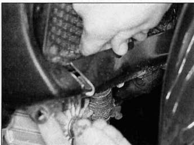
6.2a Separate the front covers from the lower cover . . .
