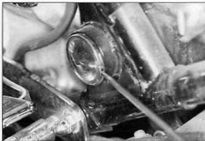
12.5 Pry out the swingarm pivot caps (there's one on each side of the bike)
