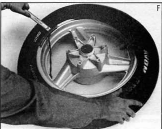
F Use a tire lever to work the second bead over rim flange.
