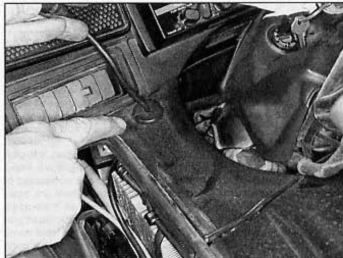
3.1c Pull the left inner fairing cover out past the accessory cable (if equipped)
