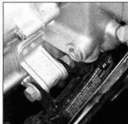
5.19 On the right side of the bike, remove the lower rear engine-to-frame bolt (shown) and the lower engine-to-frame bolt that's beneath the cylinder head
