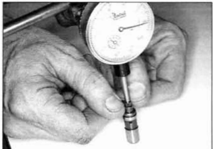
9.38 Pump the adjuster and measure its travel with a dial indicator
