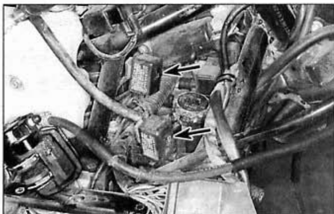
10.3 The turn signal and hazard relays (arrows) are interchangeable
