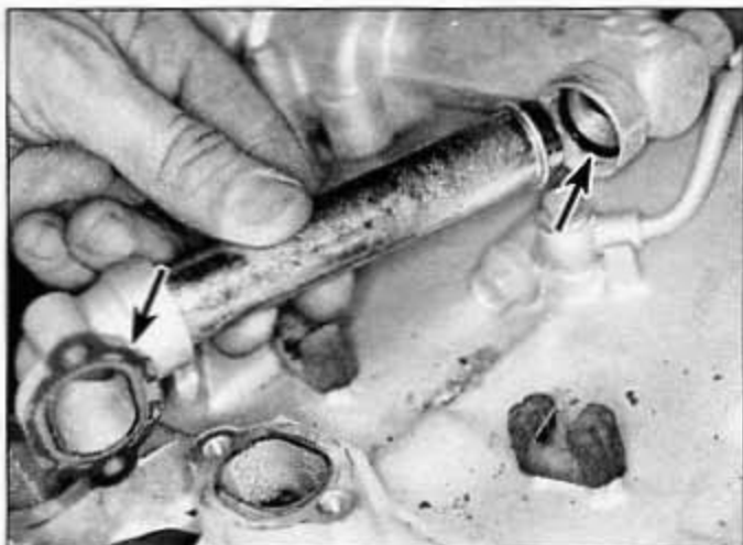
9.3 Use new gaskets and O-rings (arrows) when reinstalling the coolant tubes
