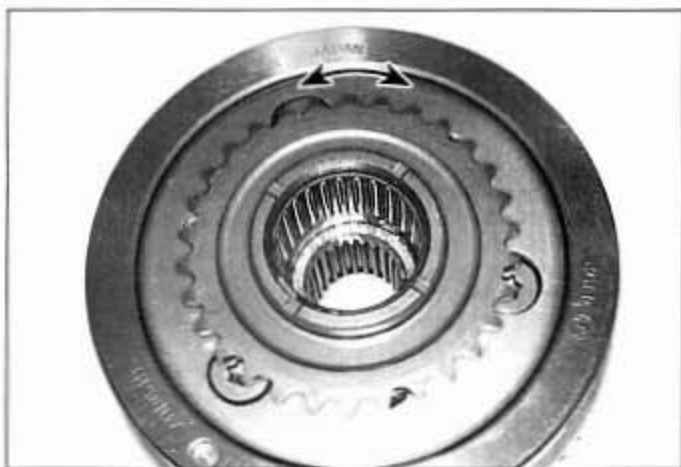
30.9b . . . and try to turn it both ways; it should turn in one direction only
