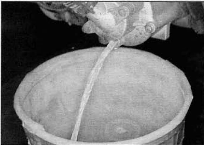
28.2 Remove the drain bolt from the water pump and let the coolant drain
