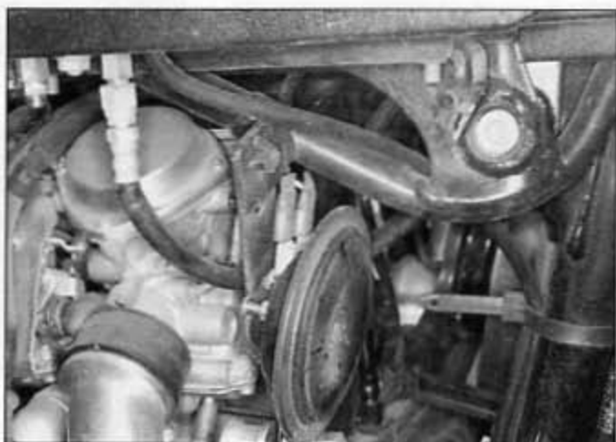
18.1 Disconnect the wires and remove the bracket bolt to detach the horn
