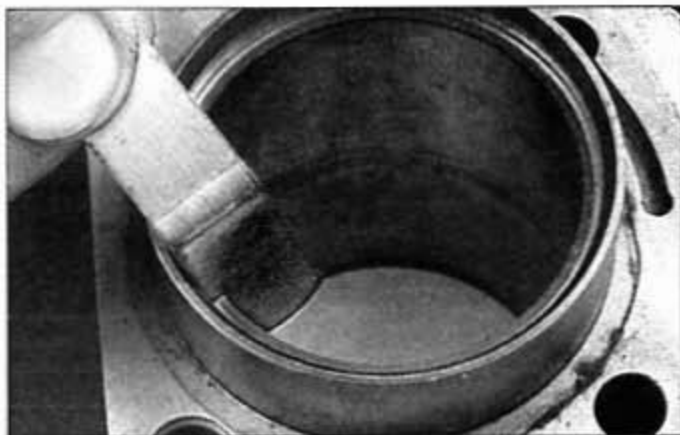
27.3 Check the ring end gap at the bottom of the cylinder
