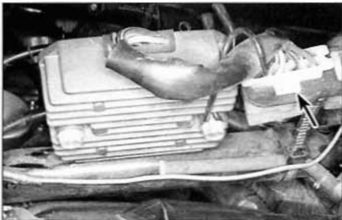
28.3 Unplug the regulator/rectifier connector at the bracket (arrow)
