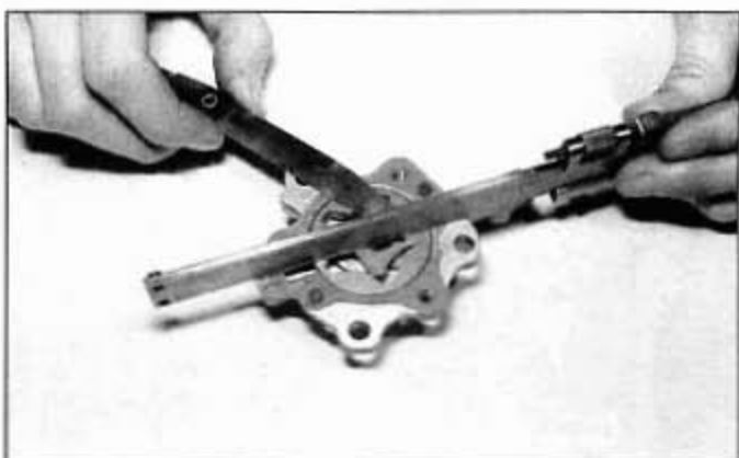
17.9c Lay a straightedge across the rotors and pump body and measure the gap
