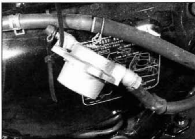
13.25 If you're removing the slave cylinder for access to other components, leave the fluid line connected and tie it up like this
