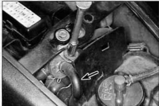
2.7 Disconnect the lower end of the hose (arrow) and remove the splash shield mounting nut
