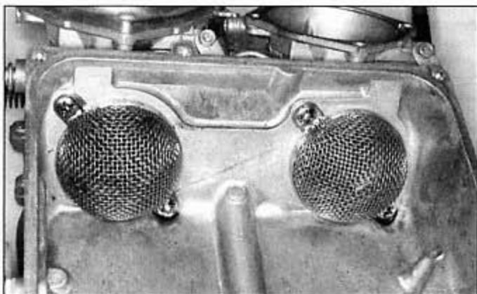
9.5a The carburetor mounting screws also secure wire screens, two on each side of the air chamber
