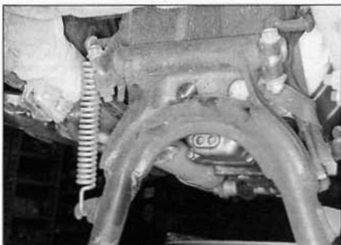
16.1c Unhook the centerstand spring and undo the clamp at each end of the pivot shaft to remove it
