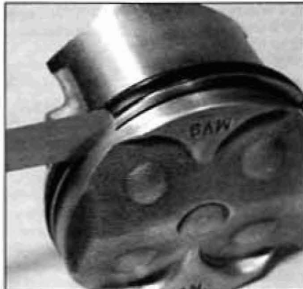
26.11 Measure the piston ring-to-groove clearance with a feeler gauge
