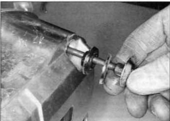
8.3b . . . and replace the rubber seals if they're brittle or deteriorated; on installation, coat the seal with oil
