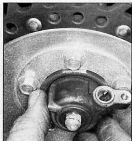
12.6 Take the speedometer drive unit off the axle
