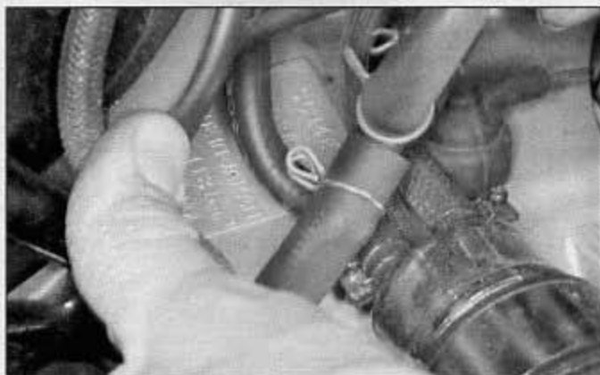
The engine number is stamped in the right side of the crankcase
