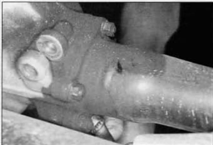
10.2 Remove the four mounting nuts; one nut is hidden behind the swingarm
