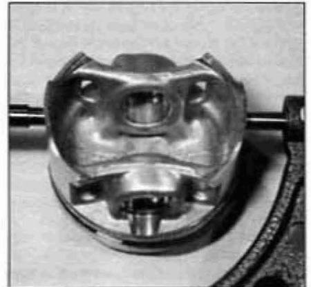
26.12 Measure the piston diameter with a micrometer
