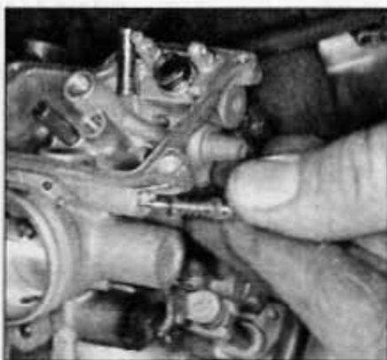
10.2d Unscrew the pilot screw all the way and pull it out, together with the spring, washer and O-ring
