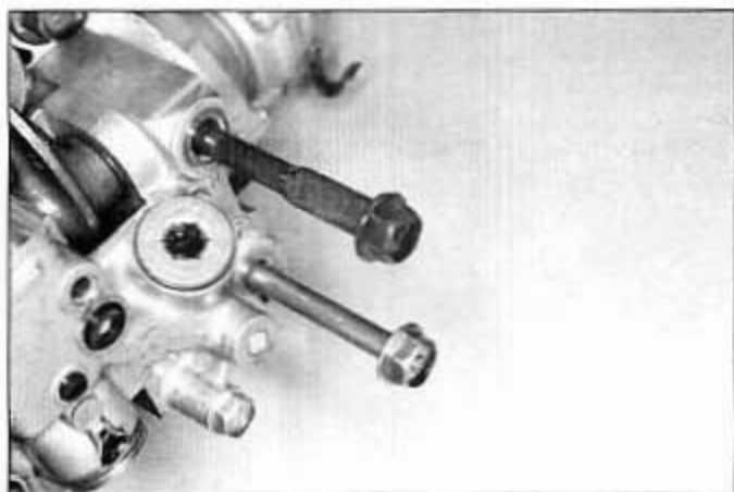
9.5b The upper camshaft holder bolts are shouldered; the lower ones are plain
