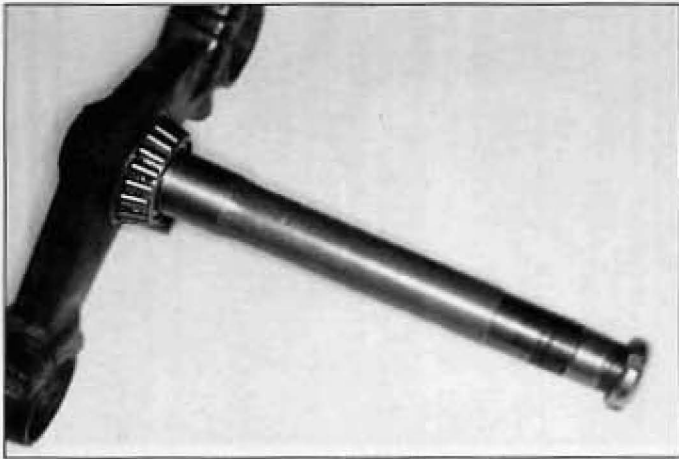
7.14a Thread the nut onto the steering stem, then clamp the nut in a vise and tap the bearing off
