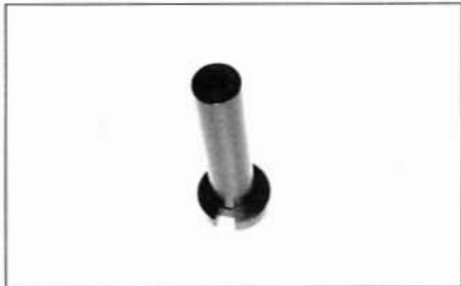
9.47a This gauge is used to select lash adjuster shims . . .
