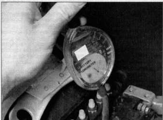
4.6 Check the specific gravity with a hydrometer
