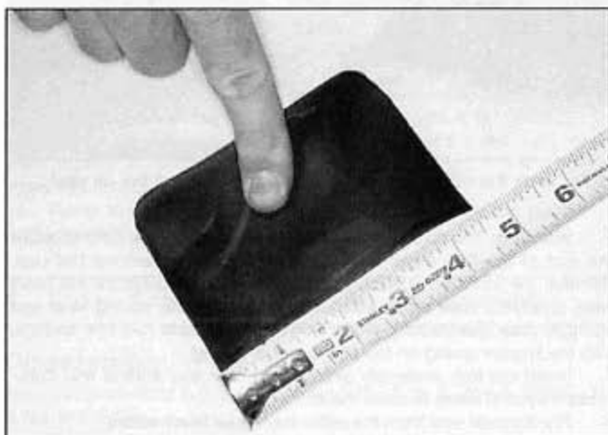
5.12a Cut a piece of soft, flexible plastic to the width shown . . .
