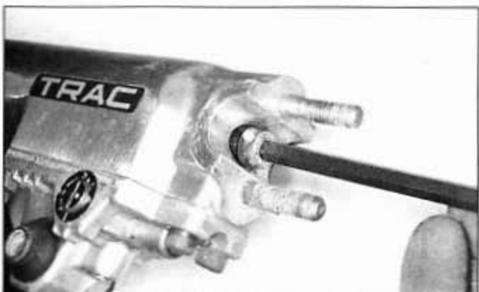
5.6a Unscrew the damper rod Allen bolt and remove the sealing washer; use a new sealing washer on assembly
