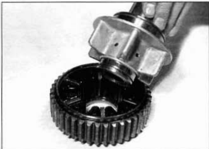
34.7b . . . and lift out the coupling for access to the rubber segments
