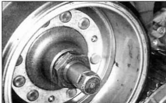
30.6b Undo the nut and washer to remove the rotor; the bolt need not be removed
