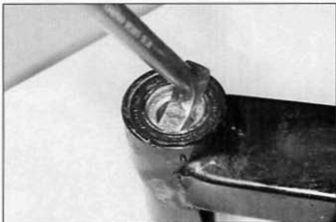
13.3a Pry the grease seal out of the swingarm; this seal remover is easy to use, but a screwdriver will also work
