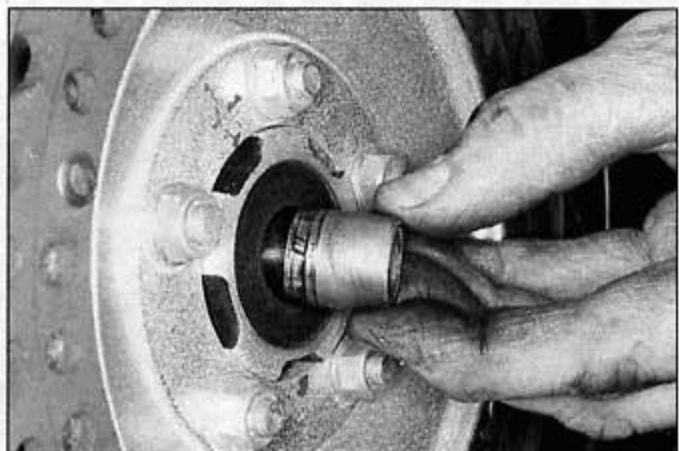
12.7 Remove the spacer from the right side of the wheel
