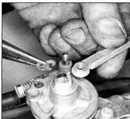
9.3 The throttle rods pivot on nylon bushings; remove the cotter pin, metal washer and nylon washer to detach the rods from the pivot
