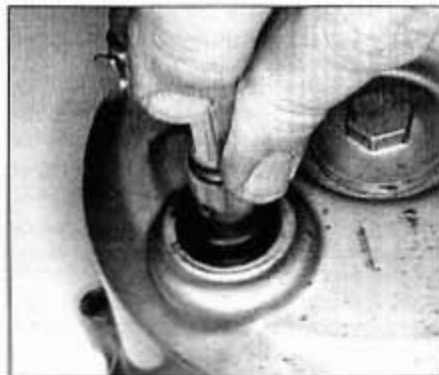
30.4a Push the grommet out of the housing with a socket
