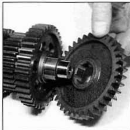
33.13c At the other end of the shaft, slide off the output gear (1984 through 1986 models)
