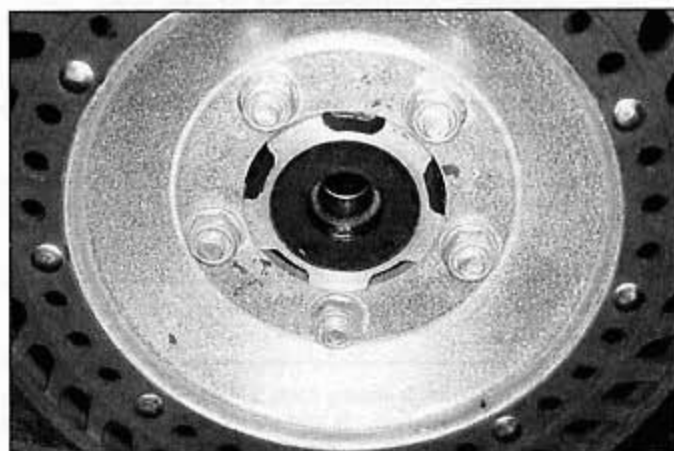
4.6 Remove the self-locking nuts and take the disc off the wheel; use new nuts on installation
