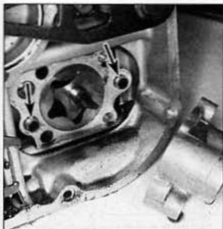
19.2b ... pull the cover off the oil pump, locate the dowels (arrows) and remove the outer rotor
