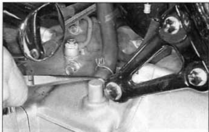
5.10 Disconnect the breather hose from the crankcase
