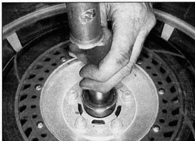
14.8 Drive in the new bearings and seals with a driver like this one or with a socket the same size as the bearing outer races
