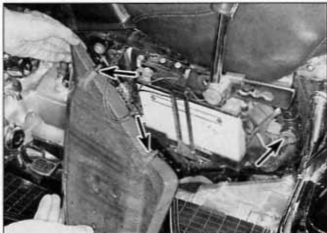
8.1 The side cover posts fit into rubber grommets (arrows)
