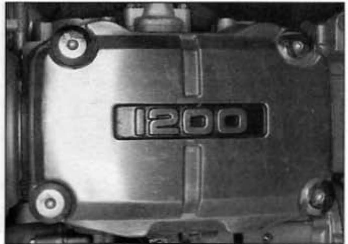
8.3a Unscrew the cover bolts (arrows) . . .
