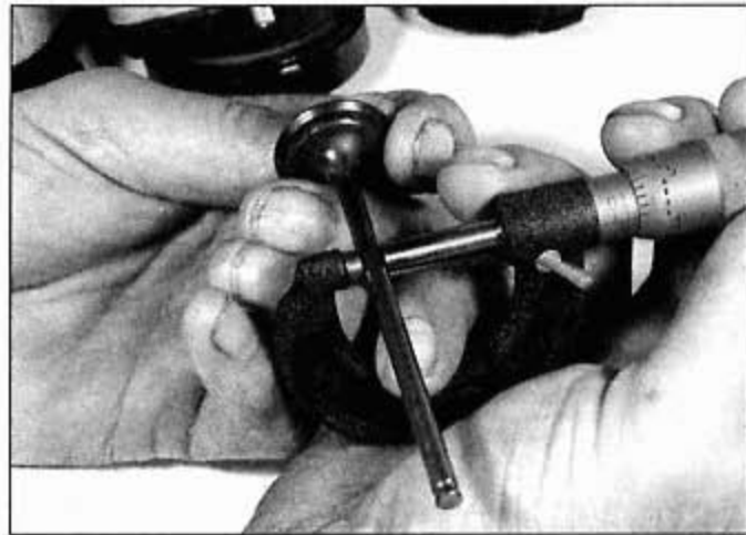
12.18a Measure the valve stem diameter with a micrometer
