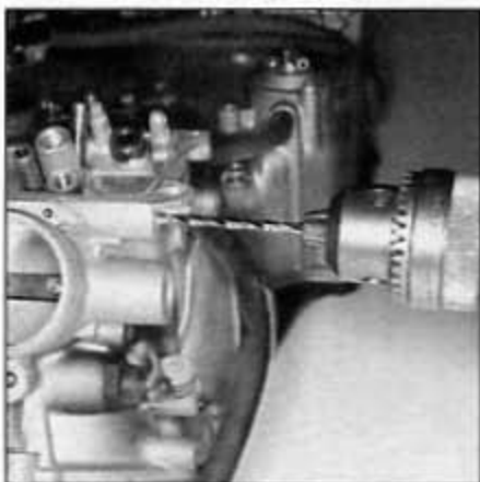
6.3a Drill a hole in the plug, but be careful not to hit the pilot screw with the drill (carburetor shown inverted)
