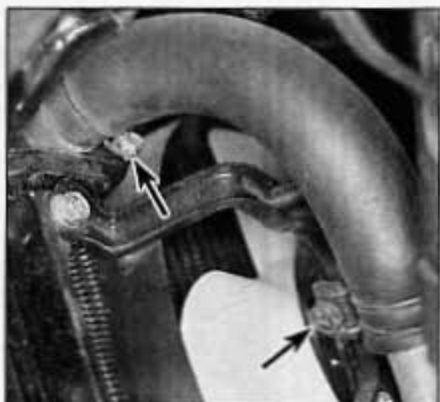
7.5a Loosen the clamp screws (arrows) and remove the upper radiator hose
