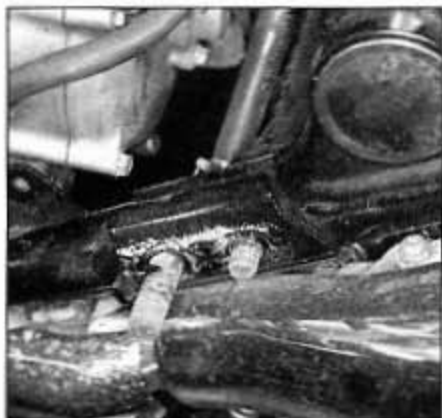
5.18b Remove the cap nuts from these studs at the rear end of the subframe . . .
