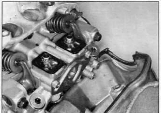
8.4 Take the cover and gasket off the cylinder head
