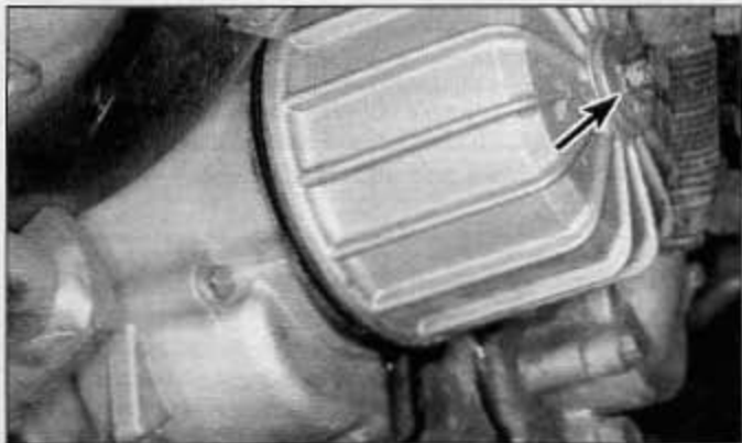
11.5a Partially loosen the oil filter bolt (arrow) and let the filter housing drain
