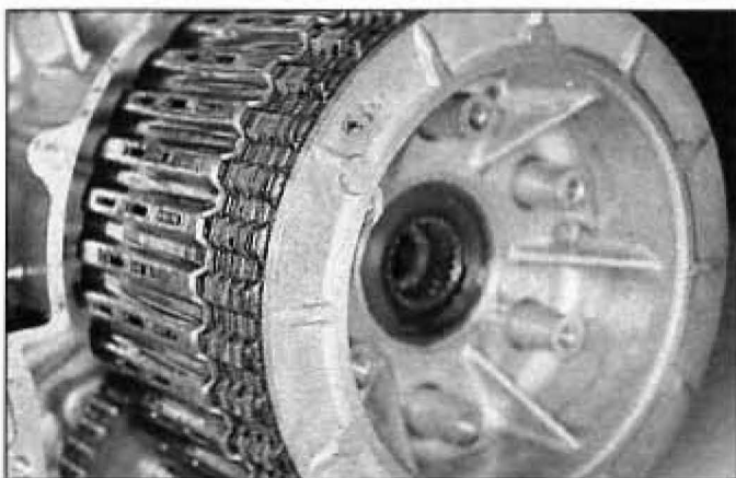
14.9 Pull the clutch center and plates off as a pack
