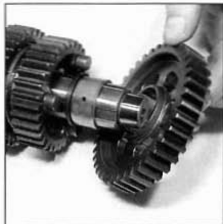
33.13d Slide off first gear . . .
