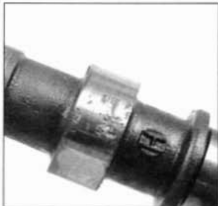
9.9a Check the lobes of the camshaft for wear - here's a good example of damage which will require replacement (or repair) of the camshaft
