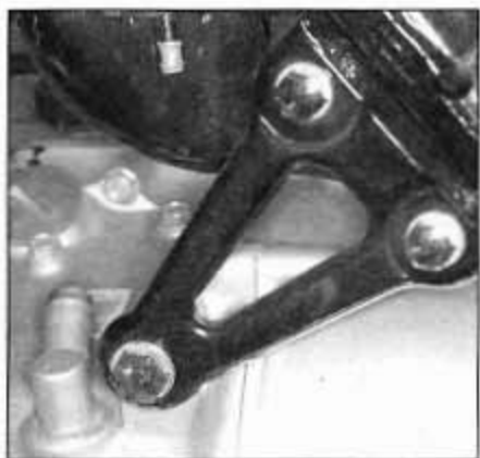
5.20b . . . remove two small bolts from the left engine mount . . .
