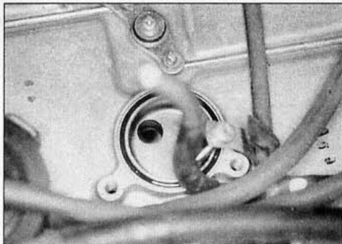
14.5e This O-ring isn't easily accessible, so it's a good idea to replace it with a new one whenever the reed case is removed
