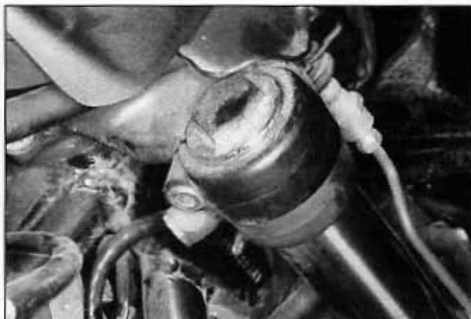
3.3 Loosen the fork cap
