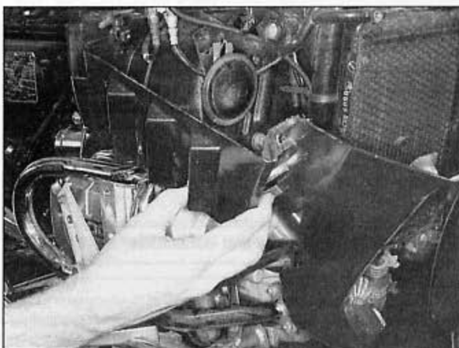
6.2b . . . and lift the front covers off the bike
