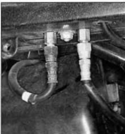
9.2a Note the different colors of the hose fittings . . .
