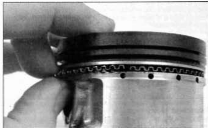
27.9a Installing the oil ring expander - make sure the ends don't overlap
