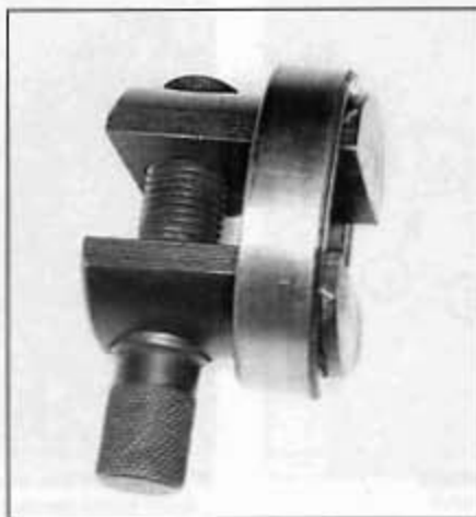
7.11b This tool is inserted into the lower race and expanded to catch its edges . . .
