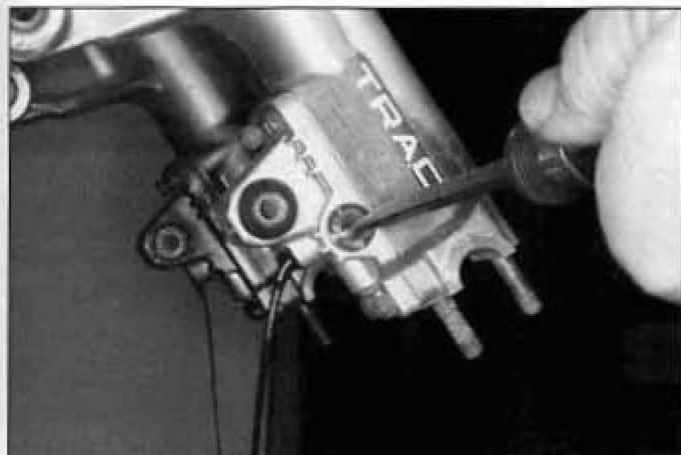
3.2 Remove the drain screw and turn the anti-dive adjuster for maximum oil flow
