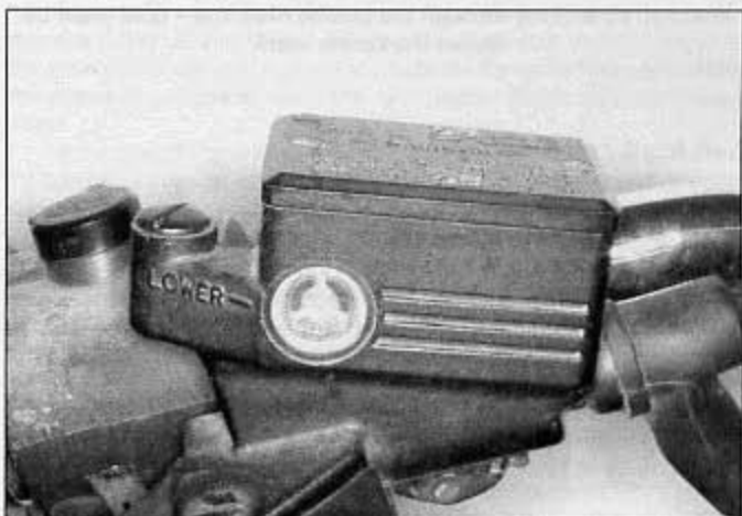
3.8a With the master cylinder in a level position, check fluid level in the inspection window (be sure the fluid level in the window is above the Lower mark) - this is the master cylinder for the right front brake . . .
