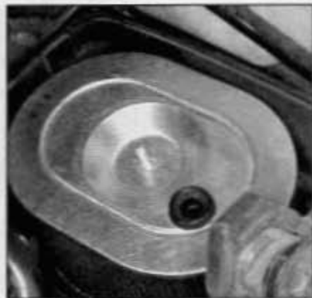
13.3c ... and lift out the element
