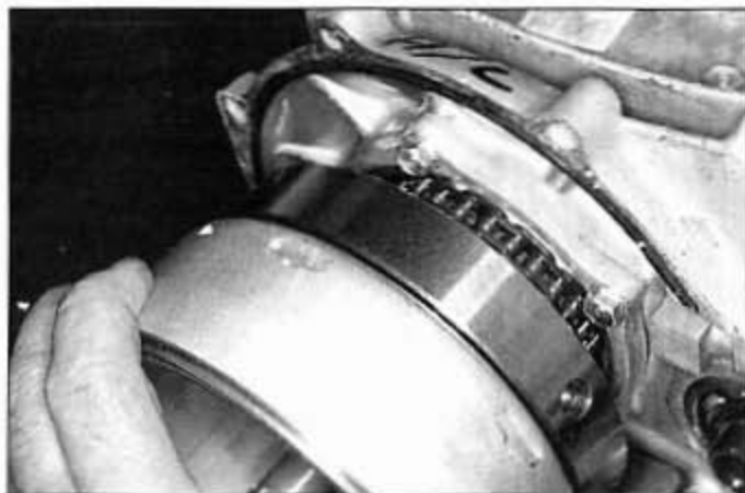
30.7 Pull the rotor and starter clutch off the shaft
