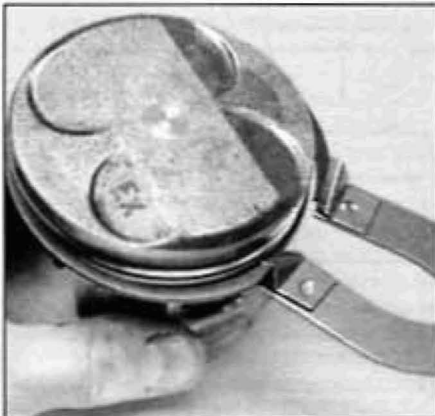
26.4 Remove the piston rings with a ring removal and installation tool
