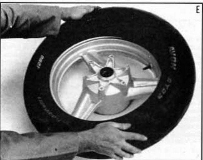
E Work first bead over the rim flange.
