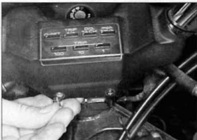
2.1 Remove the screws and lift the cover off the handlebars; if the cover includes the keyboard shown here, turn it over and unplug the wiring connector
